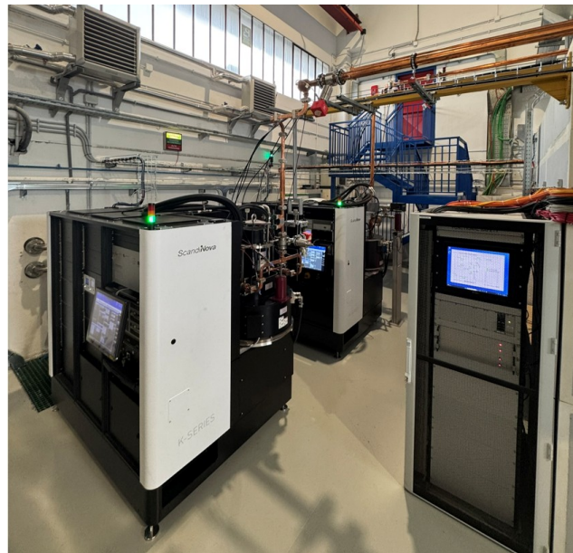
Figure 2: The 25MW X-band source and the 22MW C-band source installed in the final position.
