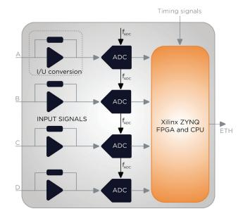
The input current is converted to voltage and amplified using a transimpedance amplifier. The ADCs sample the data and provide the output to the FPGA.
