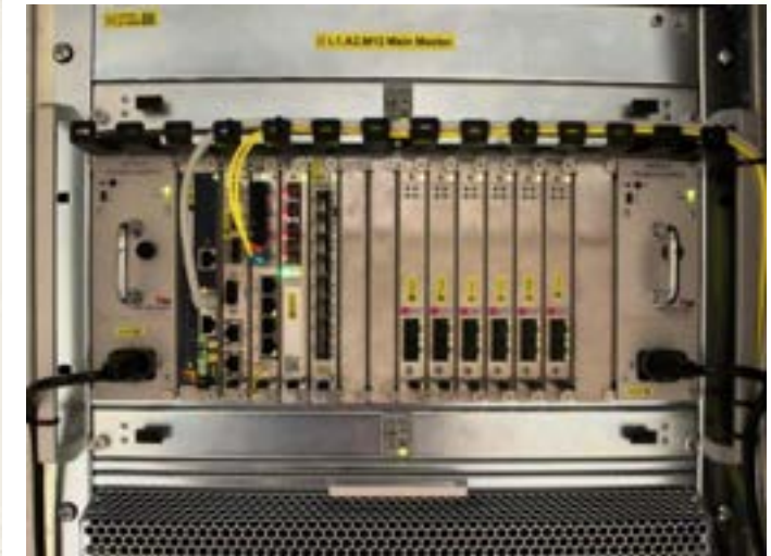
DESY's in-house developed MTCA.4-based LLRF system.
