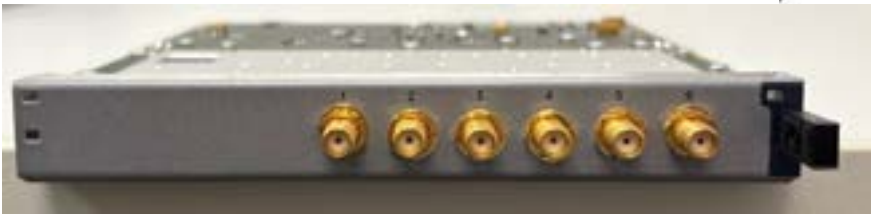
New generation 6 channel KADC module based on Xilinx KUP technology.
