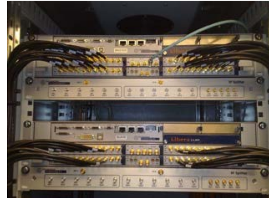
EMMA FFAG Libera LLRF installation (2010): 19 cavity vector sum control
