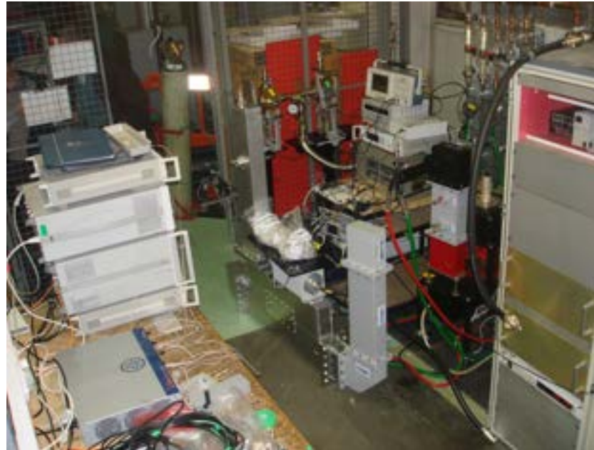
Libera LLRF high-power bench testing
