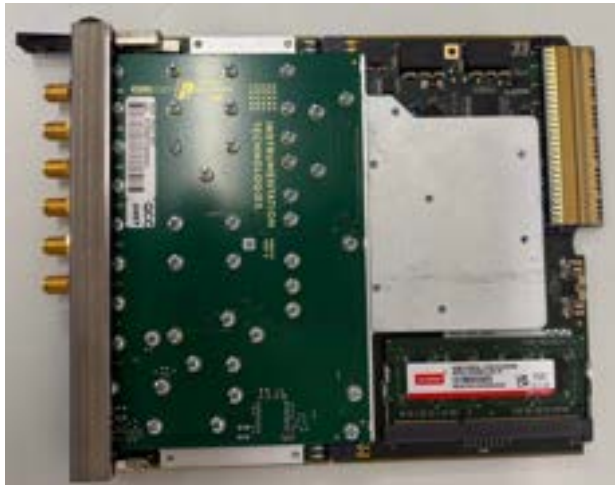
New generation 6 channel KADC module based on Xilinx KUP technology.
