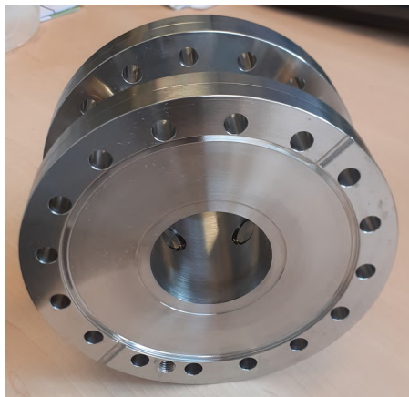
Figure 4: Beamline BPM by NTG. Aperture 50 mm, button diameter 12 mm, total length 80 mm, DN100CF.
