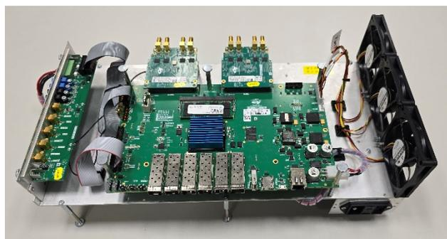
Figure 3: DAQ manufacturing test stand.
