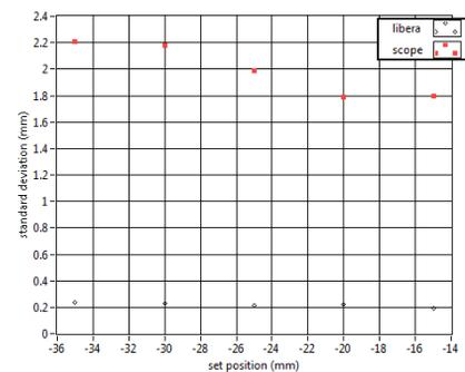
Figure 4: Standard deviation for CNAO front end and Libera (on X axis there is set position in mm and on Y axis standard deviation).
