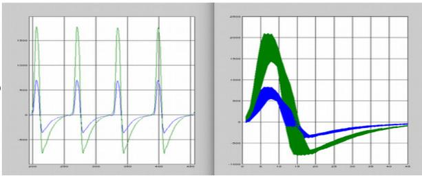
Figure 5: Left plot presents digitalized signals A and C directly from pickup. Extracted bunch informations from 1 ms data acquisition (ADC data) is presented on the right plot (~1900 extracted bunch signals are plotted).
