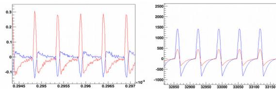
Figure 2: Sigma (red) and Delta (blue) acquired by the CNAO front end electronics (left figure). Right (red) and Left (blue) electrodes acquired by the Libera electronics.
