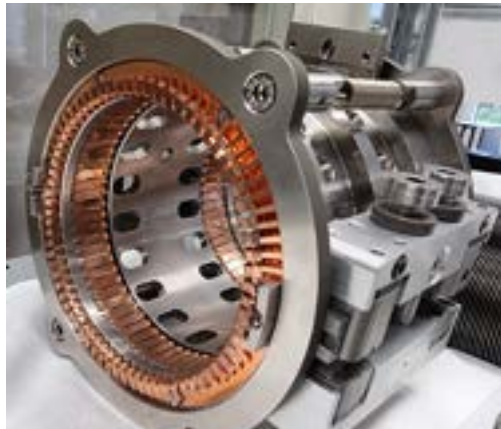
Figure 4: RF cage that is being moved into position if the viewers are not used. Once in its position the Copper-Beryllium springs will be moved outwards to insure a good electric conductivity. This is done in order to minimize the overall impedance of the storage ring.
