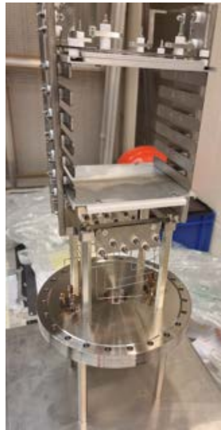
Figure 3: The ready mounted vacuum part of the IPM. On top a module with a MCP stack and a phosphor screen will be mounted. The E-field-box with its 6 field flattening electrodes is visible. On the bottom, covered with a protective shield during mounting, a fine mesh will be installed, which flattens the electric field but lets through UV light for calibration purposes. The UV light will be generated by a lamp mounted outside the vacuum, right behind the vacuum window in the lower CF flange.
