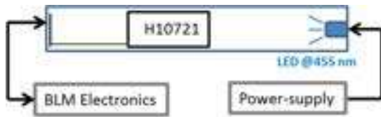
Figure 3: Setup for the calibration with a diode.
