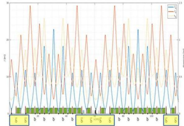
Figure 1: Booster low emittance optics.
