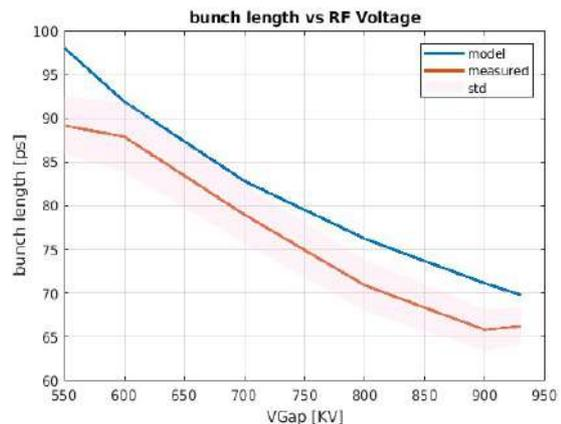
Figure 2: model vs measured bunch length.
