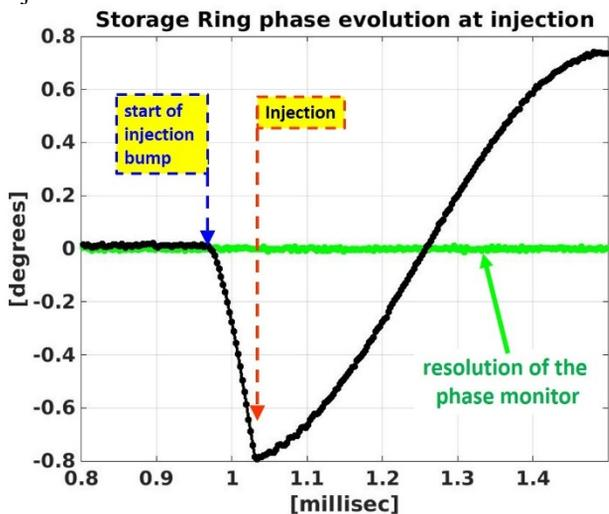
Figure 4: Details of time-resolved phase at injection.
