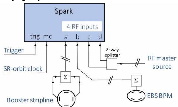
Figure 1: The connections of the phase-monitor.
