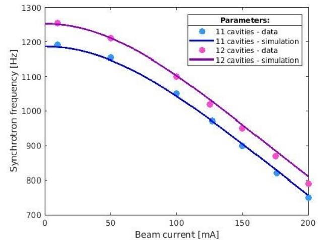
Figure 6: Simulation and measurement results of the synchrotron frequency as a function of beam current.
