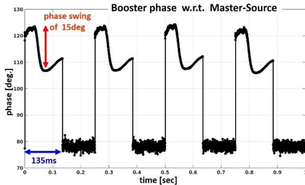
Figure 7: The time-resolved Booster-phase evolution of 4 consecutive injection cycles.
