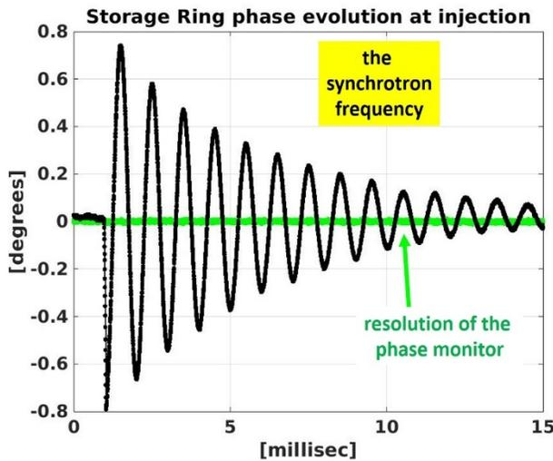
Figure 3: The time-resolved phase at injection.
