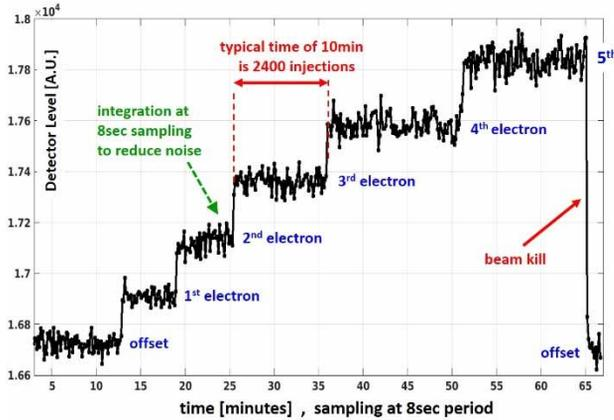
Figure 9: The injection of 1-2-3-4-5 electrons over a time span of 1 hour, measured with 8 sec integration mode.
