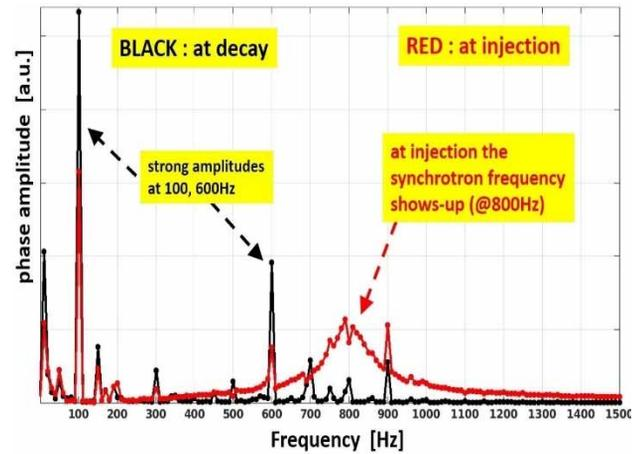
Figure 5: Frequency spectra of the phase, both at injection (red) and during normal decay (black).
