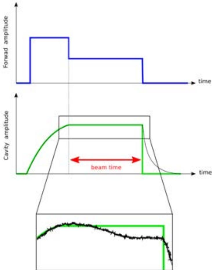
No matter how precise we are setting the pulse shape, the system variations over time and temperature will require us to use a **feedback loop** to improve the regulation
