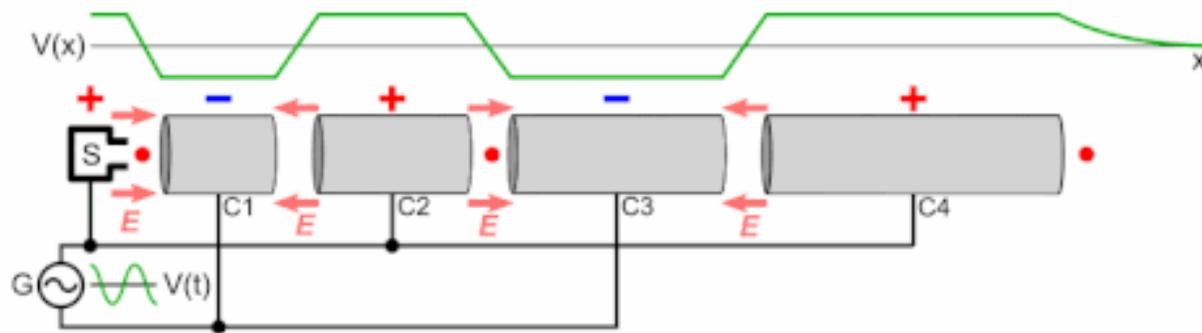
**Principle:** alternating the Electrical field across multiple plates along the particle accelerator.
