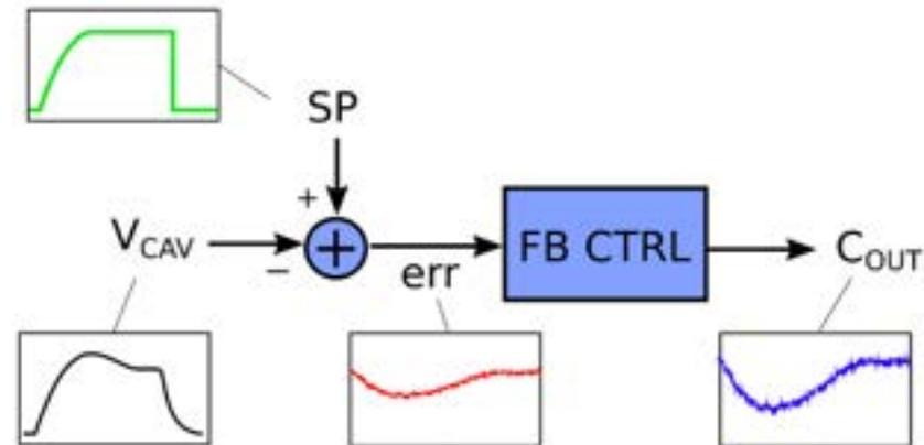
We are very interested to maintain a certain **amplitude and phase stability (RMS)** within the pulse and from pulse to pulse. Both in short term (seconds) and on long-term (hours)
