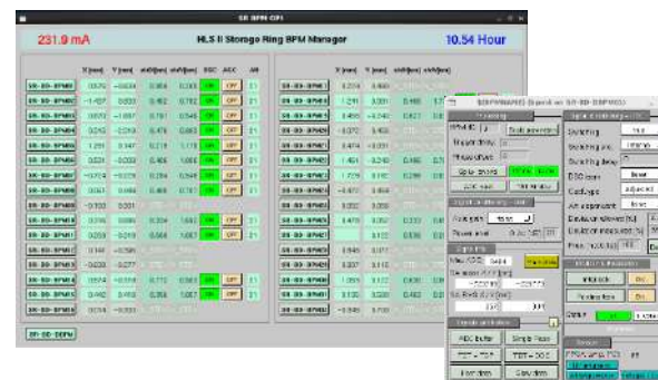
Interface of the BPM control system and OPI for one module of the Libera Brillianceplus coded by edm.
