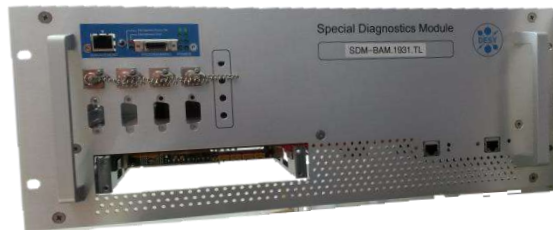
Generalized layout of special diagnostics modules, here for BAM application, with free slot for TMCB
