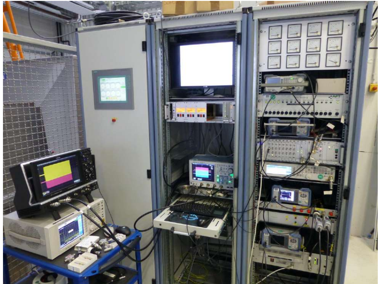
Resonant Frequency Control with stepper motor controllers, ARC detection system, fast interlock system and measurement, master oscillator, power meters and 300 W klystron driver
