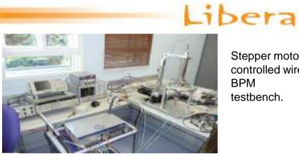
Stepper motor controlled wire BPM testbench.
