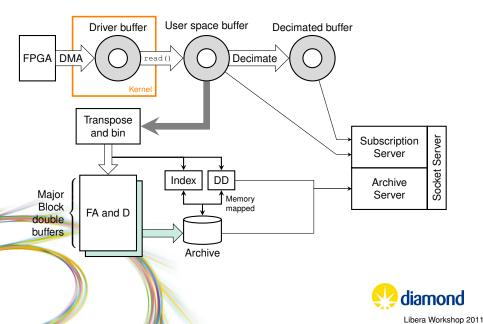
The FA archiver provides the following data over TCP/IP to any connecting machine:
