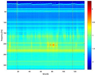
log10 vertical amplitude on BPM3-2 [log10(um)]
