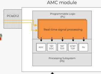
The real-time signal processing is implemented in the FPGA in the AMC module. The memory buffers are dedicated for turn-by-turn, multi-bunch turn-by-turn, raw ADC and other data paths.
