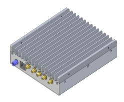
Libera Pilot Tone FE combines the RF and pilot-tone signals at the BPM pickup of electron synchrotrons. Drifts of the cables between the Libera Pilot Tone FE and BPM electronics are compensated by the digital algorithm.
