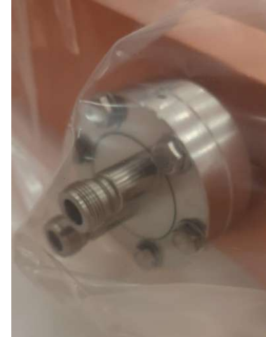
Directional Coupler for the VEGA Injector System. RF connector: N-type, 50 ohms.
