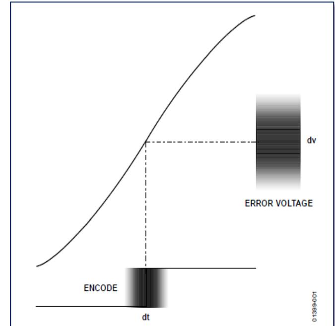
Noise induced by jitter:  $V_{err} = 2\pi \cdot A \cdot f \cdot t_{jit}$
