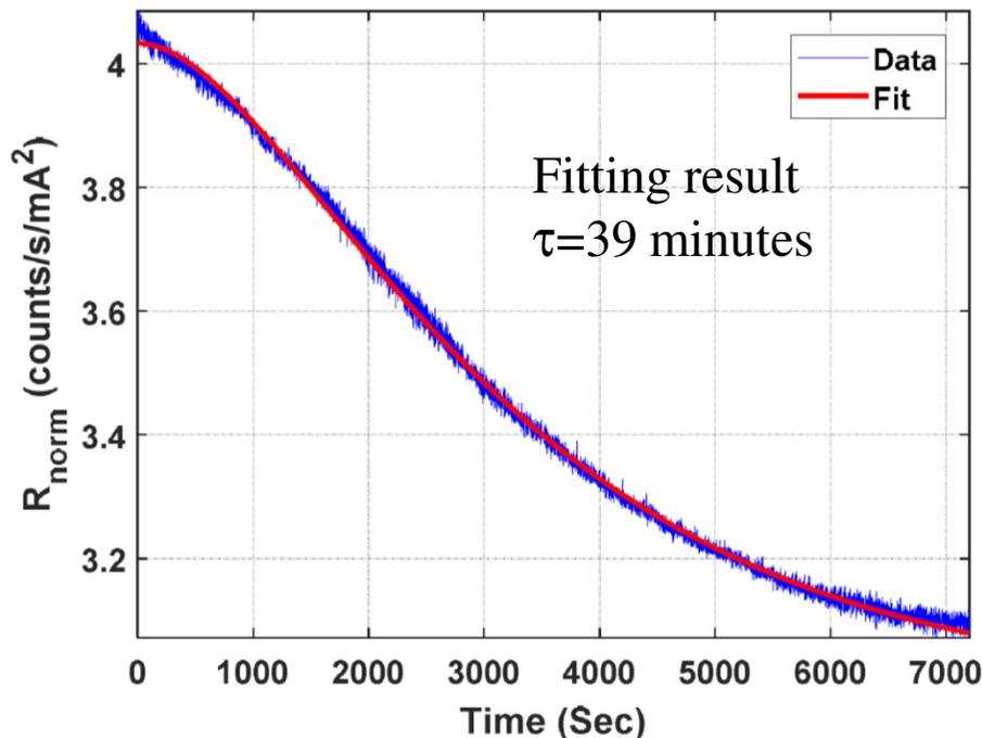
For TPS, the operating energy ( $E$ ) is 3 GeV,  $\rho$  is 8.40 m,  $R$  is 82.5 m and the polarization time is around 40 minutes.
