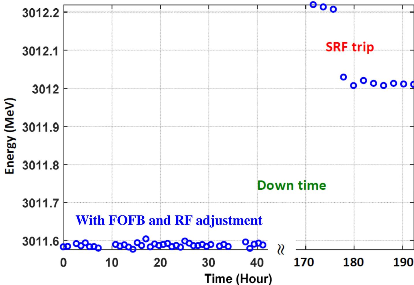
The beam energy stability measured by resonant spin depolarization is less than 20 keV ( $\Delta E/E \sim 7 \cdot 10^{-5}$ ) during continuous operation.
