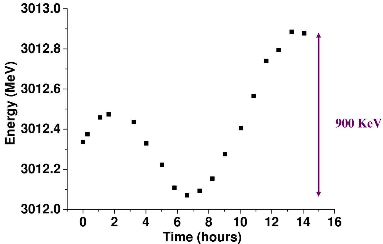
**The energy variation without feedback is much higher than with feedback and RF adjustment.**
