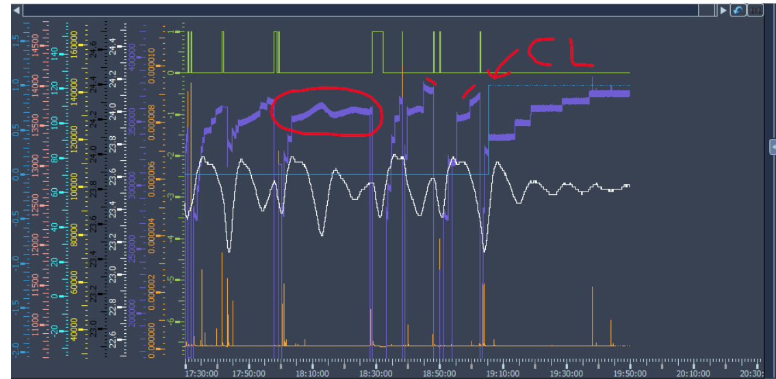
RFQ voltage (purple) during a test where cooling (white) was oscillating excessively. Once feedback control loop (cyan) was activated, stability improved.
