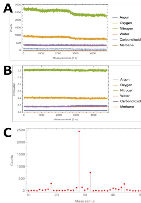
**Figure 4. Major Constituents Analysis (MCA) performed on the TB. (A) Counts vs. time; (B) frac vs. time; (C) centroid.**
