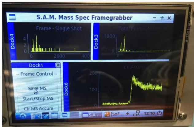
**Figure 6. Mass Spectra Shown on the DM Display.** Initial mass spectra (of residual air in chamber) with the DM operated remotely (via WiFi).
