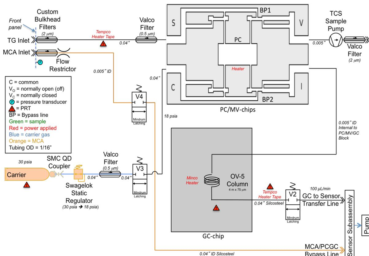
**Figure 2. Functional Block Diagram of the S.A.M.** This diagram shows the plumbing for both the Trace Gas (TG) and Major Constituents Analysis (MCA) lines. The three PCGC chips are actually housed in a single three-layer Vespel block.
