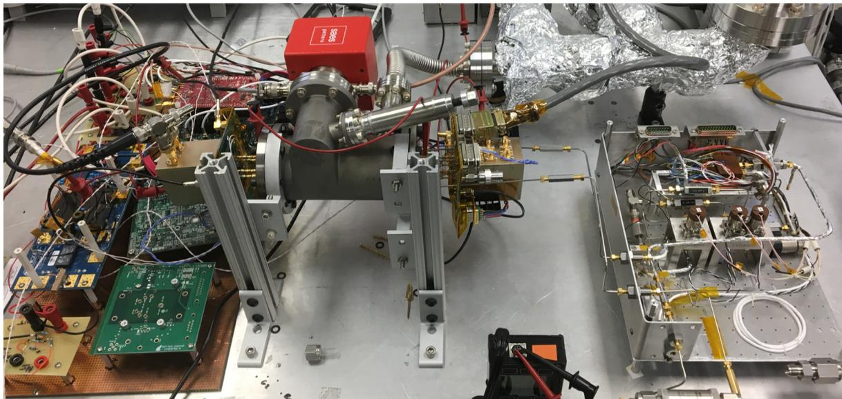
**Figure 3. Photograph of the Testbed (TB) flat-sat setup.** Breadboard electronics are on the left, the QITMS subassembly is in the middle and the PCGC subassembly is to the right.
