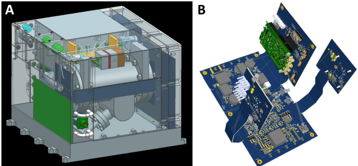
**Figure 1. Conceptual design of S. A. M. instrument.** (A) CAD model of the Spacecraft Atmosphere Monitor and (B) its flex-electronics shown separately.
