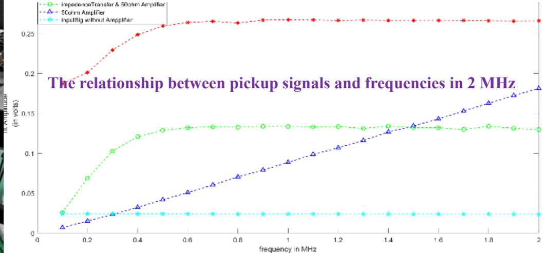
**The relationship between pickup signals and frequencies in 2 MHz**
