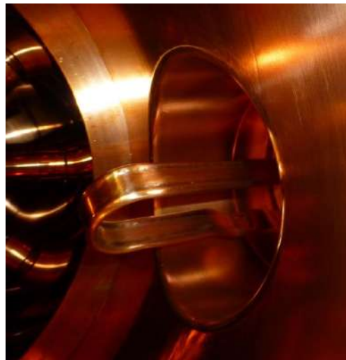
CH Cavity after copper plating at GSI (in-house)
