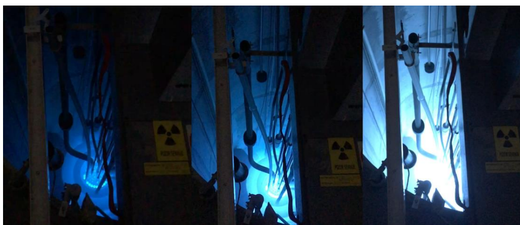
Figure 1: Sequence of three photographs taken from the reactor platform during a pulse.
