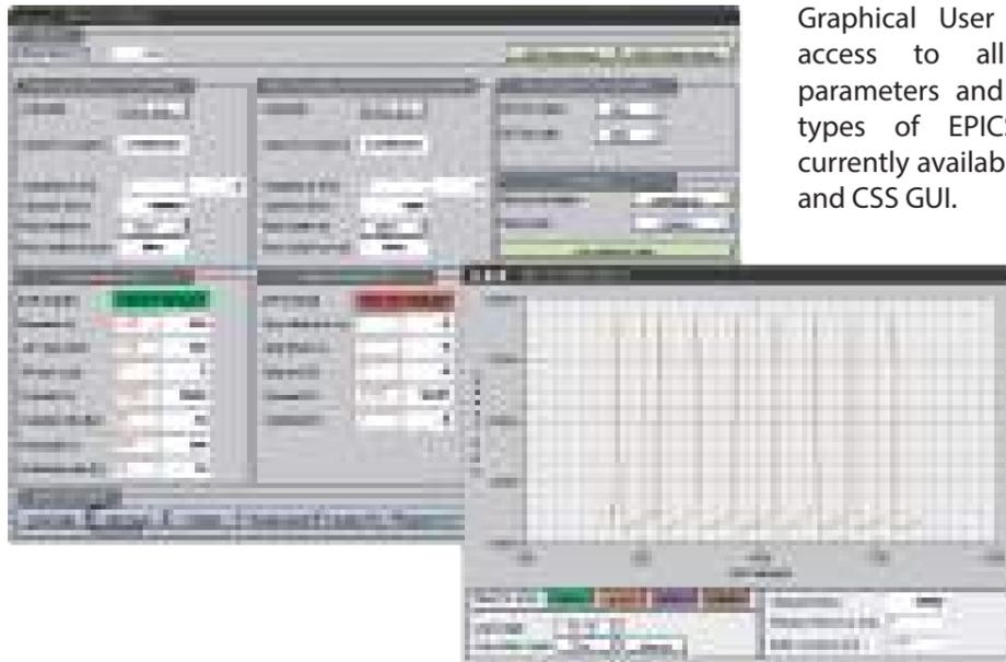
Graphical User Interfaces provide access to all the instrument parameters and signal data. Three types of EPICS-based GUIs are currently available: EDM GUI, Qt GUI, and CSS GUI.
