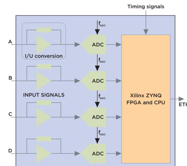
Input currents are converted into voltage via a trans-impedance amplifier, with six different gains depending on the current range selected via software. The signals are then digitized using 18-bit and 2 MSPS A/D converters (sampling frequency can be increased up to 2.5 MSPS). Offsets and gain errors can be calibrated for each channel using a nominal current source.
