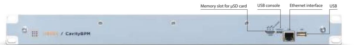
Figure 9: CavityBPM electronics based on Libera integrated platform, back panel
