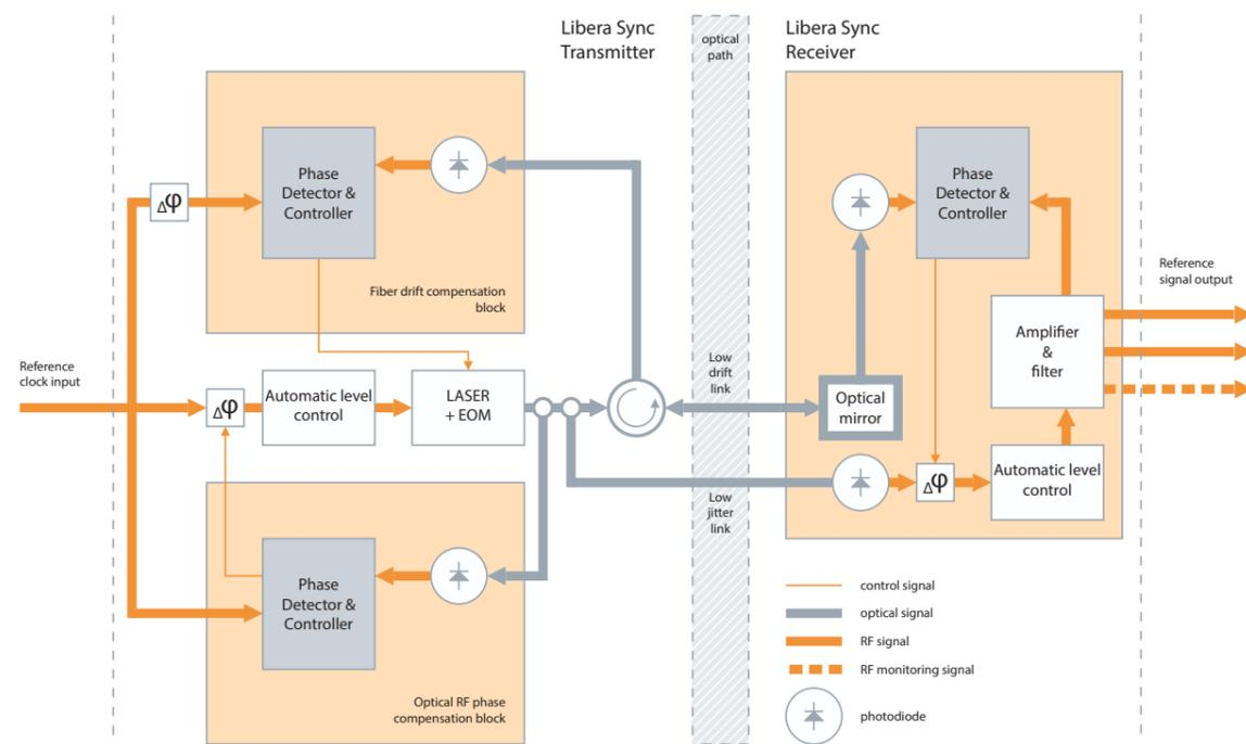
To achieve the required performance and stability over the long term, both transmitter and receiver units must be installed in an environment controlled for both temperature and humidity. Once tuned, the system requires very low maintenance.
