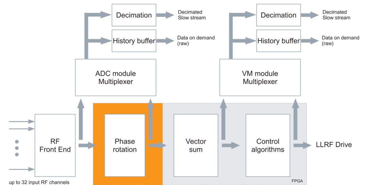
The phase rotation block is used to calibrate each different input signal in phase and amplitude; this is so that differences in RF cabling and delays resulting from the beam time of flight don't influence the calculation. The vector sum then combines all the acquired signals into one equivalent signal, which is used as the input for the control algorithm.
