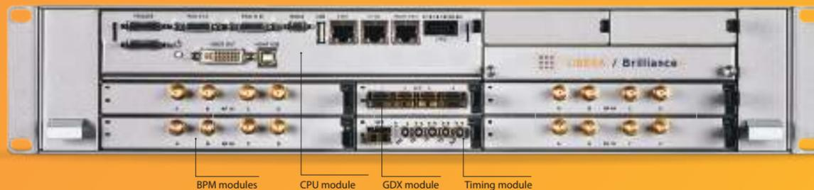
Our integrated platform is based on system-on-chip technology. Due to its low power consumption, the instrument is powered over Ethernet with PoE standard, and is passively cooled. Given the small dimension (BPM electronics is contained in a 1U 9.5" chassis), it can be installed in the tunnel close to the BPM pickup in an appropriate radiation protected location (see Figure 6).
