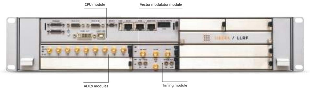
Up to four processing modules (ADC9) can be connected to the system in order to acquire up to 32 RF signals from the cavities; if less signals need to be acquired, the number of ADC9 modules can be reduced.
