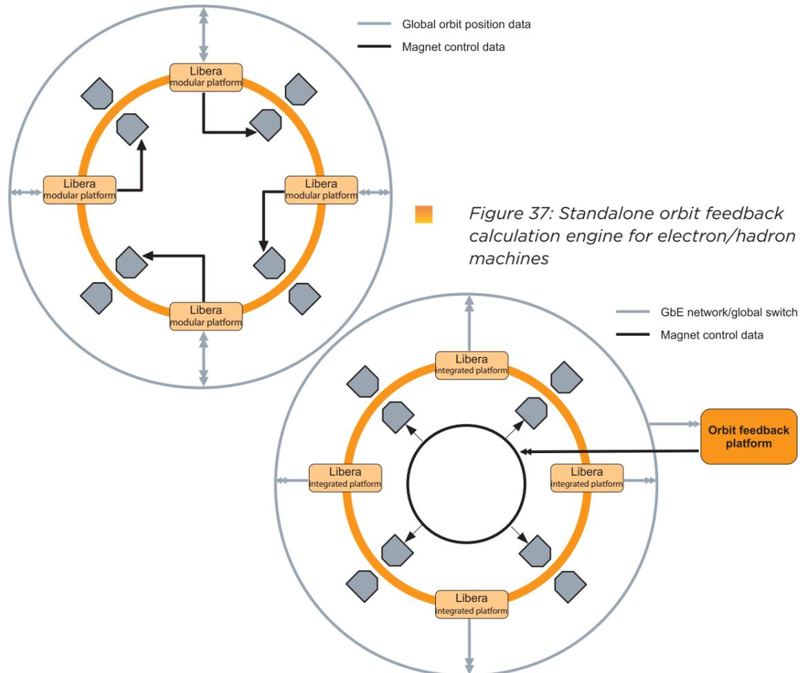
Figure 37: Standalone orbit feedback calculation engine for electron/hadron machines
