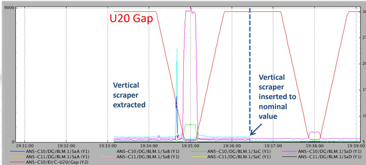
Losses measurement (SA data) on the BLM located downstream U20 in SDC10 when closing its gap.
