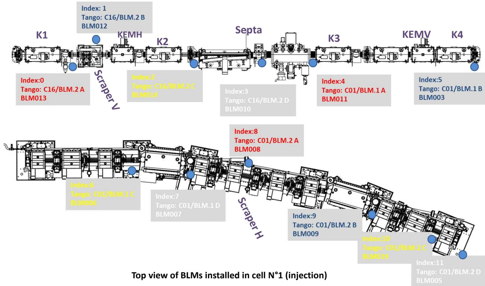
Top view of BLMs installed in cell N°1 (injection)
