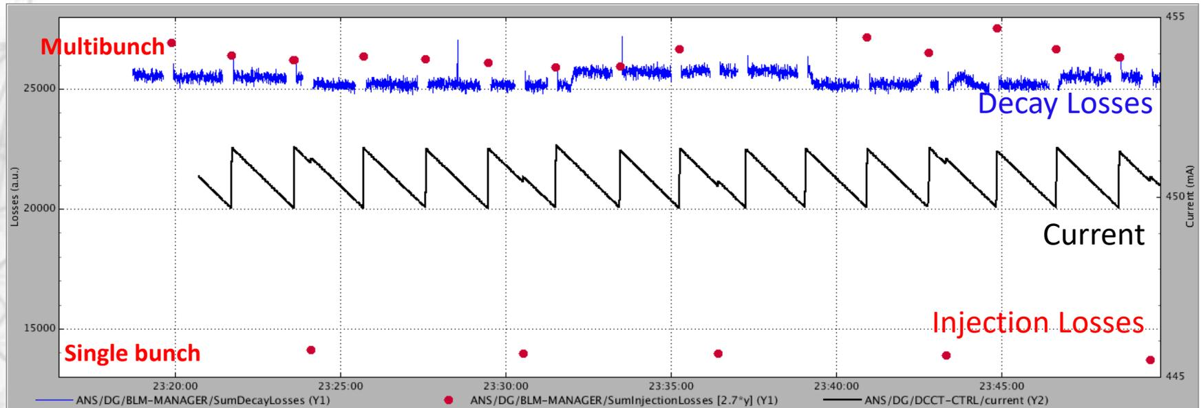
Sum of the losses during the decay of the beam (SA data in blue) and at each injection (average data, red) during hybrid filling pattern operation.
