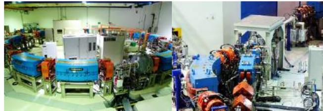
1.2 GeV synchrotron booster and storage ring
