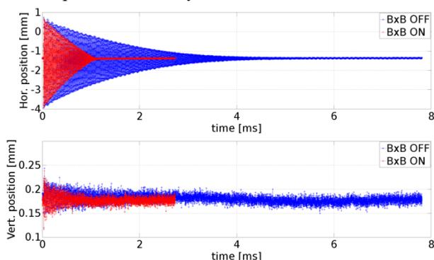
Figure 9: Damping time with BxB feedback ON / OFF.
