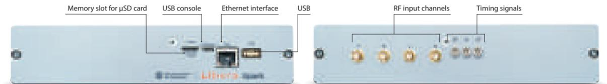
Photon BPM electronics is still based on Platform C and provides a second RJ-45 interface that is used to output the Fast data stream and a USB port. TRIAX connectors are used for input channels (Figure 7).
