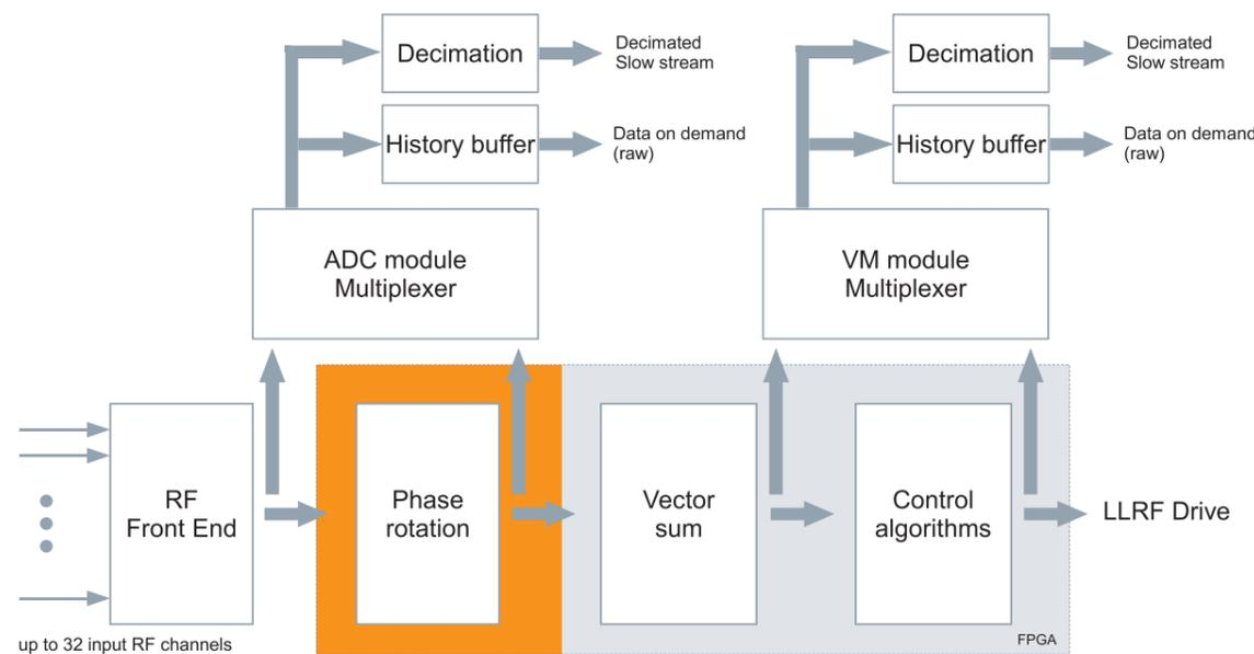
The phase rotation block is used to calibrate each different input signal in phase and amplitude; this is so that differences in RF cabling and delays resulting from the beam time of flight don't influence the calculation. The vector sum then combines all the acquired signals into one equivalent signal, which is used as the input for the control algorithm.
