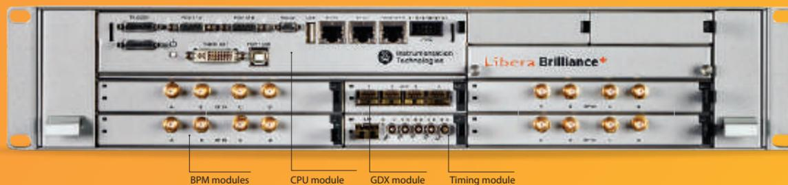
Platform C is based on system-on-chip technology. Due to its low power consumption, the instrument is powered over Ethernet with PoE standard, and is passively cooled. Given the small dimension (BPM electronics is contained in a 1U 9.5" chassis), it can be installed in the tunnel close to the BPM pickup in an appropriate radiation protected location (see Figure 6).
