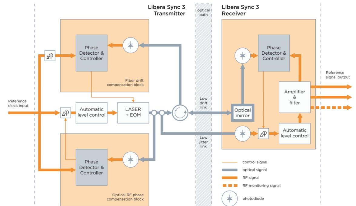
To achieve the required performance and stability over the long term, both transmitter and receiver units must be installed in an environment controlled for both temperature and humidity. Once tuned, the system requires very low maintenance.
