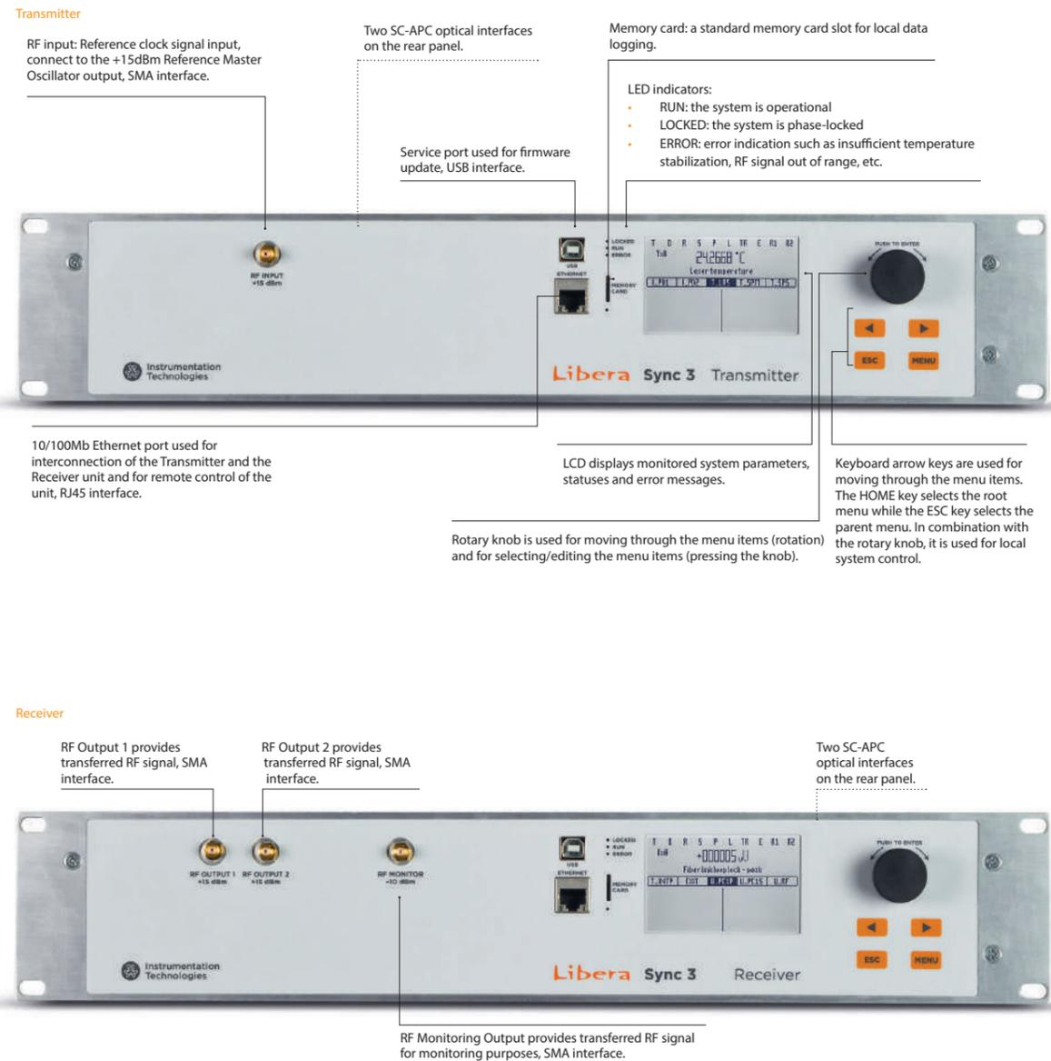
The transmitter input signal is a continuous wave RF reference signal that modulates an optical carrier through an electro-optical modulator. The modulated signal is split into two parts and fed into the two optical links: a low-drift link and a low-jitter link (see the block scheme in Figure 19). The low-drift signal is partially reflected at the receiver and is used to perform phase drift compensations in the transmitter.
