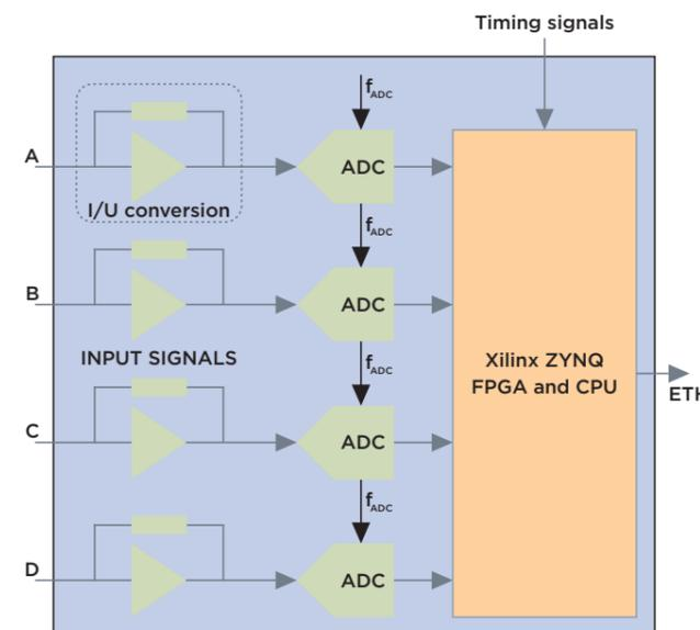
Input currents are converted into voltage via a trans-impedance amplifier, with six different gains depending on the current range selected via software. The signals are then digitized using 18-bit and 2.5 MSPS A/D converters. Offsets and gain errors can be calibrated for each channel using a nominal current source.
