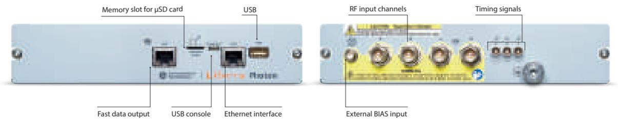
The BPM electronics for the cavity-type BPM pickups are also based on Platform C, which in this case is enlarged to a 1U 19" chassis due to the higher amount of heat that needs to be passively dissipated. The instrument can be expanded to four RF inputs and SFP connectors for fast data exchange.
