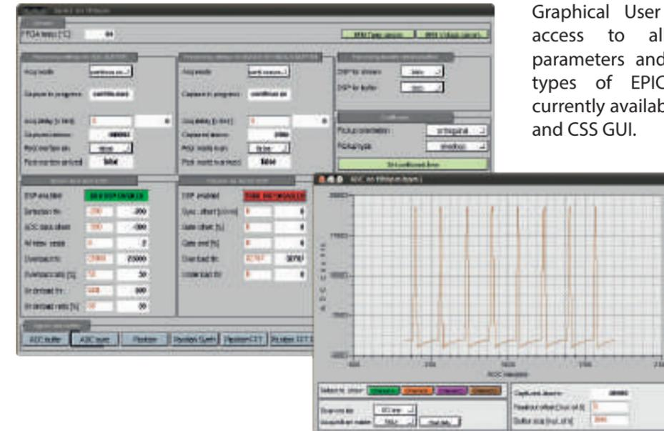
Graphical User Interfaces provide access to all the instrument parameters and signal data. Three types of EPICS-based GUIs are currently available: EDM GUI, Qt GUI, and CSS GUI.
