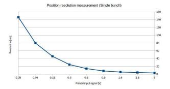
Figure 4: Single bunch measurement performance versus input signal level (0 dBFS = 5 V peak).
