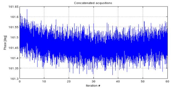
**Figure 5: Long term acquisition over 1 minute; 120us window was acquired every second at 1MS/s rate.**
