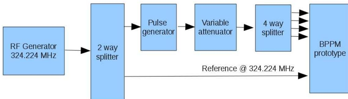
**Figure 2: Setup of the measuring chain**
