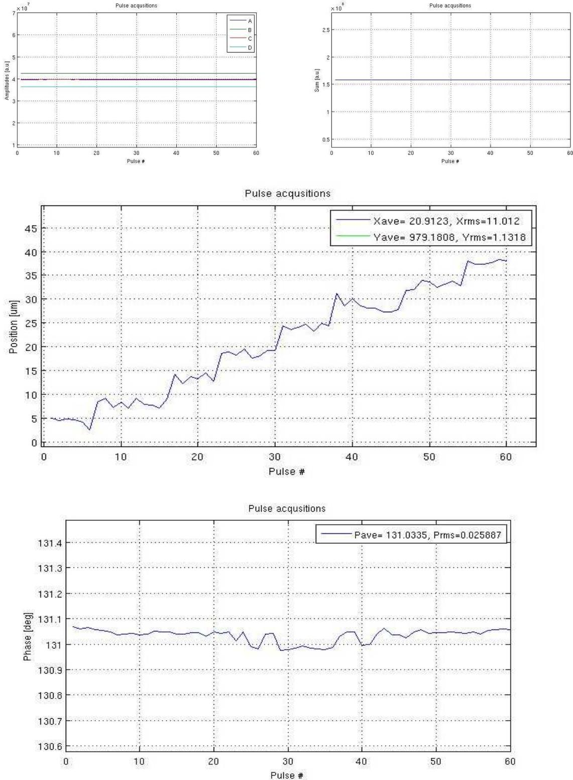
**Figure 8: Wire movement – by 5  $\mu\text{m}$  steps in x-direction. 7 steps are seen in position measurement .**
