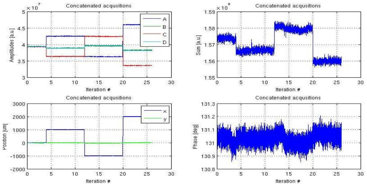
**Figure 7: Measurements of wire positions at a large scale ( $x = 0$  mm,  $+1$  mm,  $-1$  mm,  $+2$  mm;  $y = 0$  mm).**
