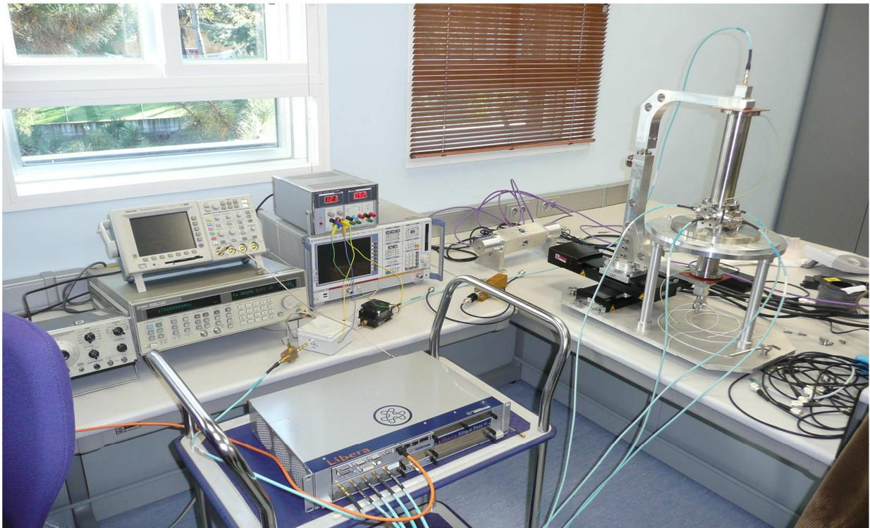
**Figure 6: Testing setup at CIEMAT: Generated signal is connected to the wire at the top of wire test bench), four button-type electrodes are connected to Libera Single Pass H (in front), just besides the reference signal input. The wire position may be controlled in X and Y by means of two stepper motors (black)**
