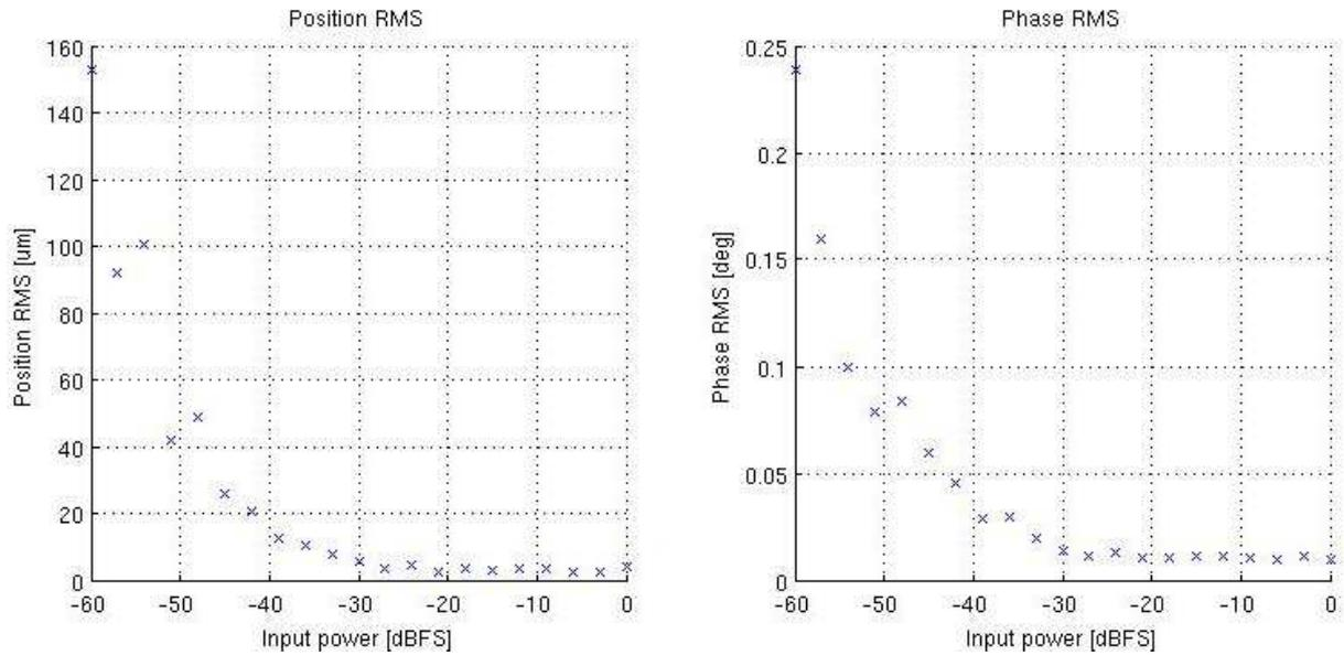
**Figure 3: Measured position and phase uncertainty in the range of 60 dB at 650 MHz (0 dBFS corresponds to  $\pm 4V$  input.)**
