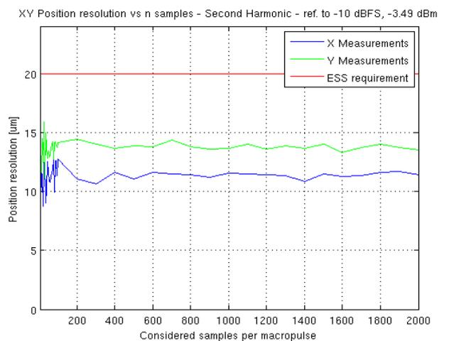
Figure 22: Position resolution dependence on number of samples per macro-pulse, -10 dBFS
