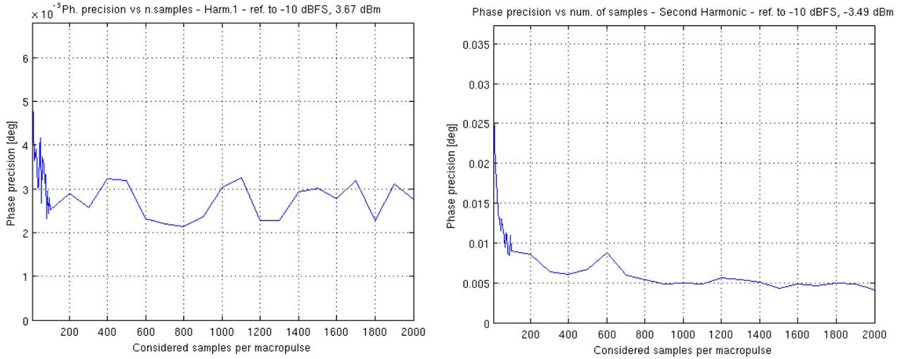
Figure 27: Phase precision dependence on number of samples per macro-pulse, -10 dBFS
