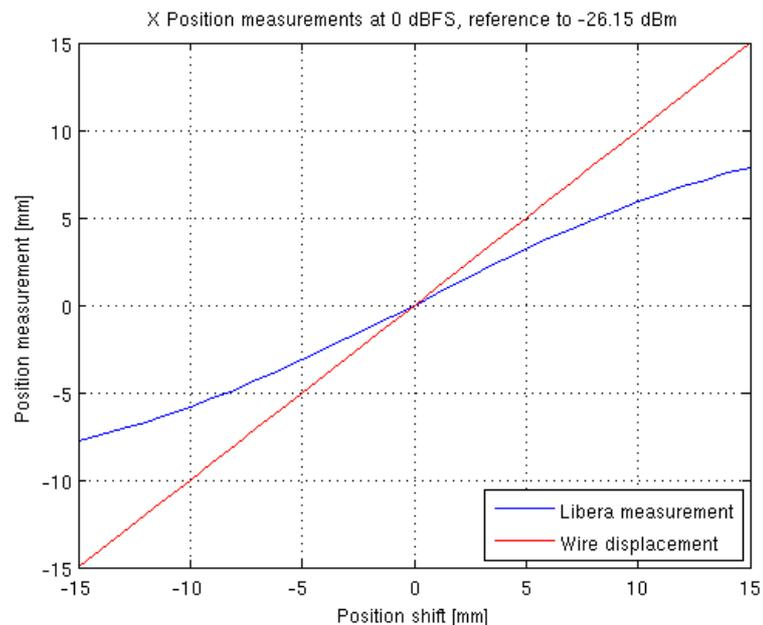
Figure 80: Position measurements after geometric calibration
