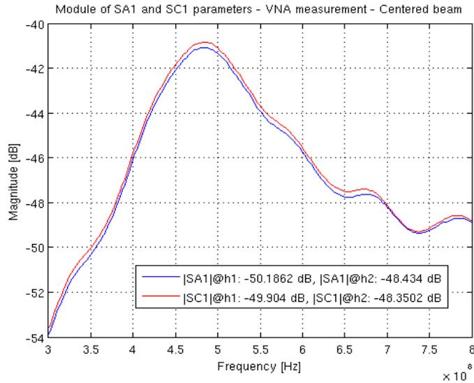
Figure 72: Modules of SA1 and SC1 with centered beam
