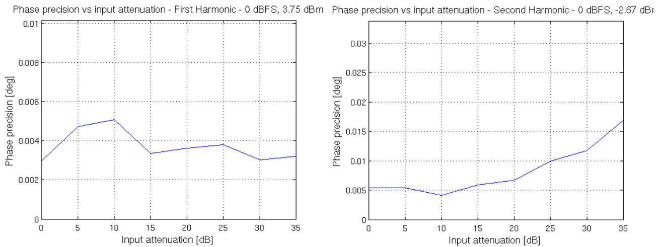
Figure 25: Phase precision dependence on the input signal level
