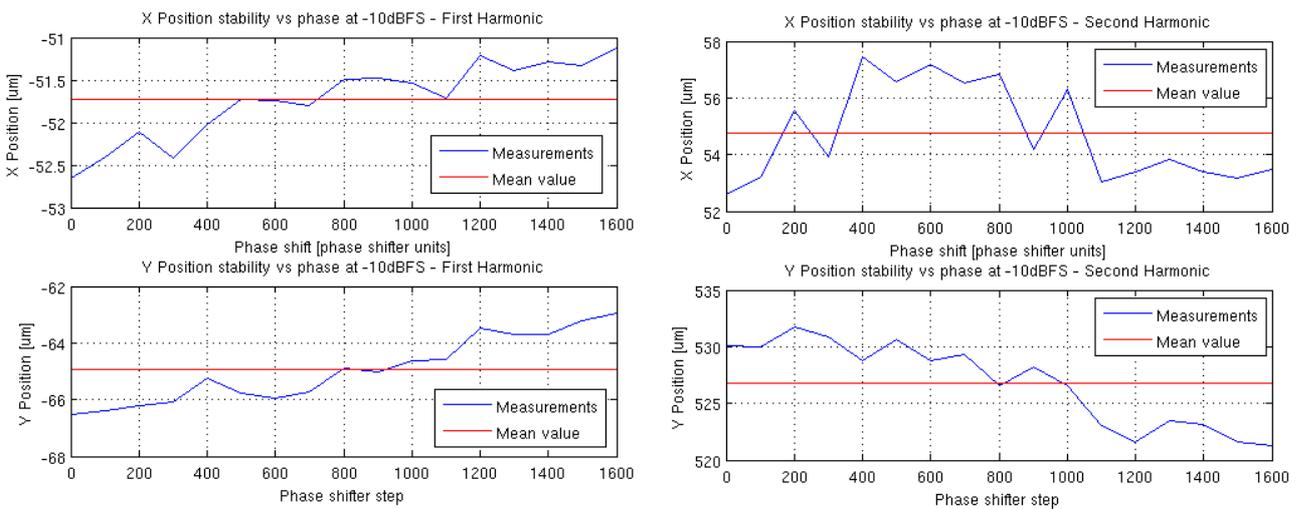
Figure 38: Position stability vs phase at -10dBFS
