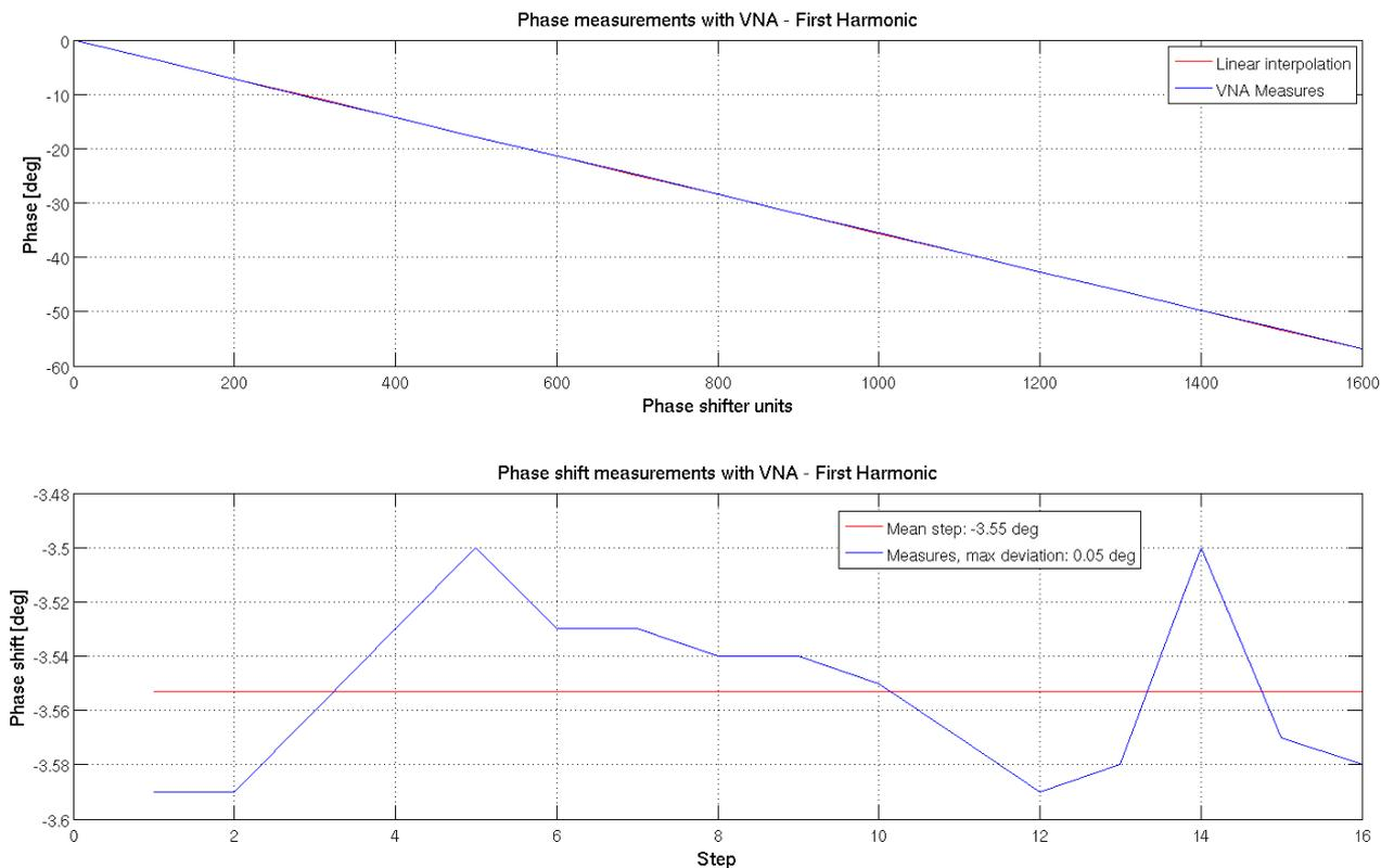
**Figure 9: Phase shifter characterization at 352.21 MHz**
