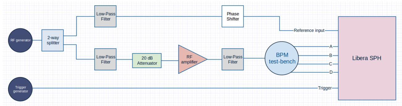
Figure 76: Test setup for measurements with the BPM test-bench
