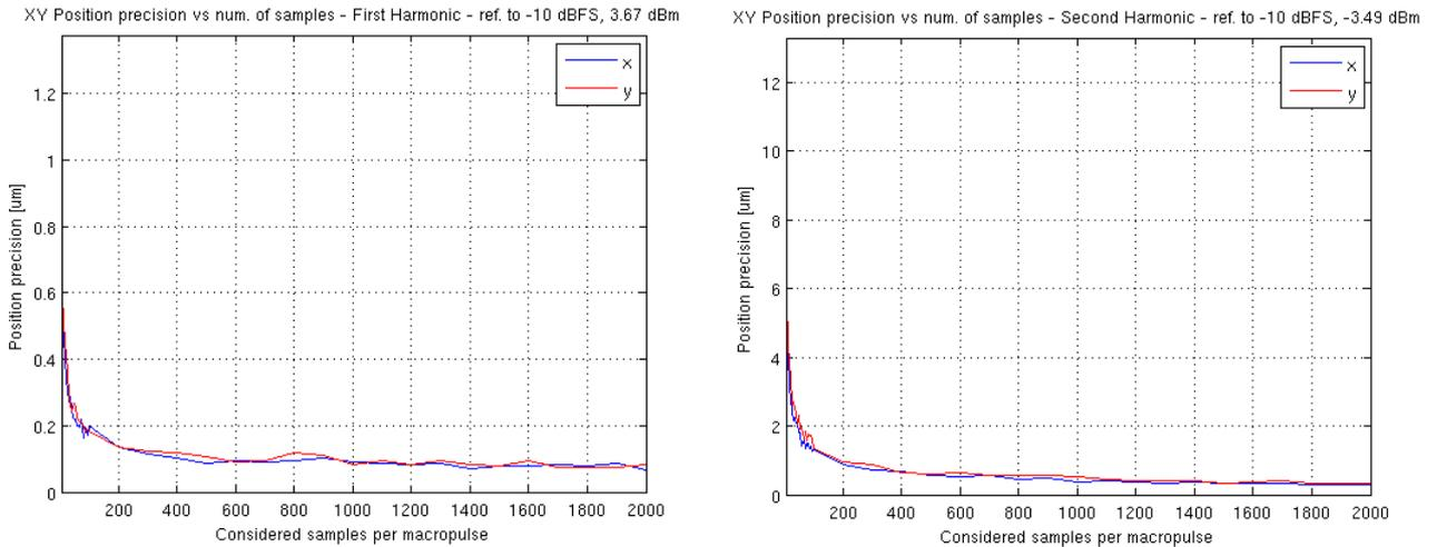
Figure 28: Position precision dependence on number of samples per macro-pulse, -10 dBFS
