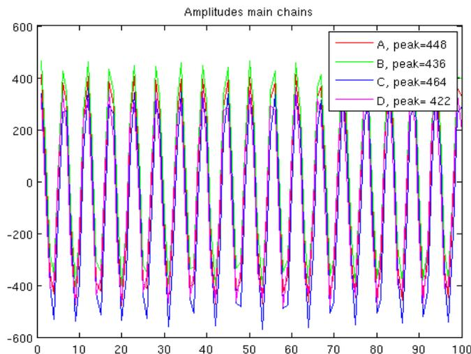
Figure 77: ADC signals from Libera SPH - Centered beam - 0dBFS
