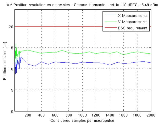
Figure 22: Position resolution dependence on number of samples per macro-pulse, -10 dBFS
