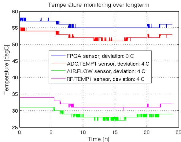
Figure 43: Temperature variation over 24h long-term test
