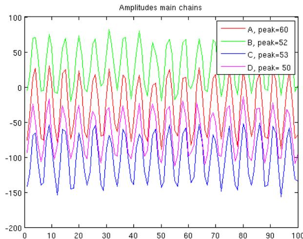
Figure 91: ADC signal levels at -20 dBFS
