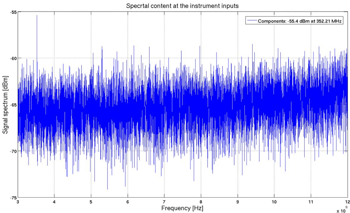
Figure 85: Spectrum of the instrument input signals at -30dBFS
