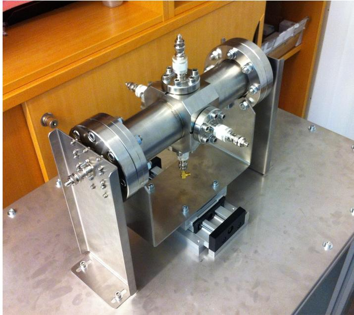
*Figure 2: BPM test bench*
