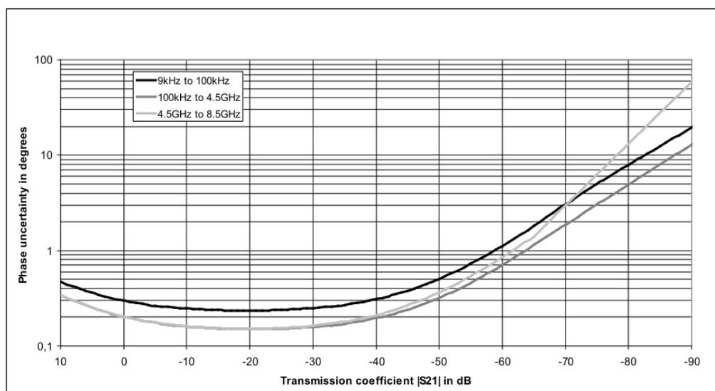
Figure 8: VNA accuracy specified by the manufacturer [5]
