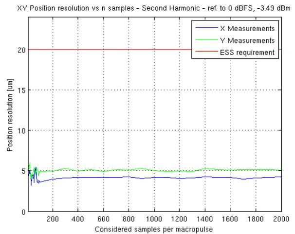
Figure 20: Position resolution dependence on number samples per macro-pulse, 0 dBFS
