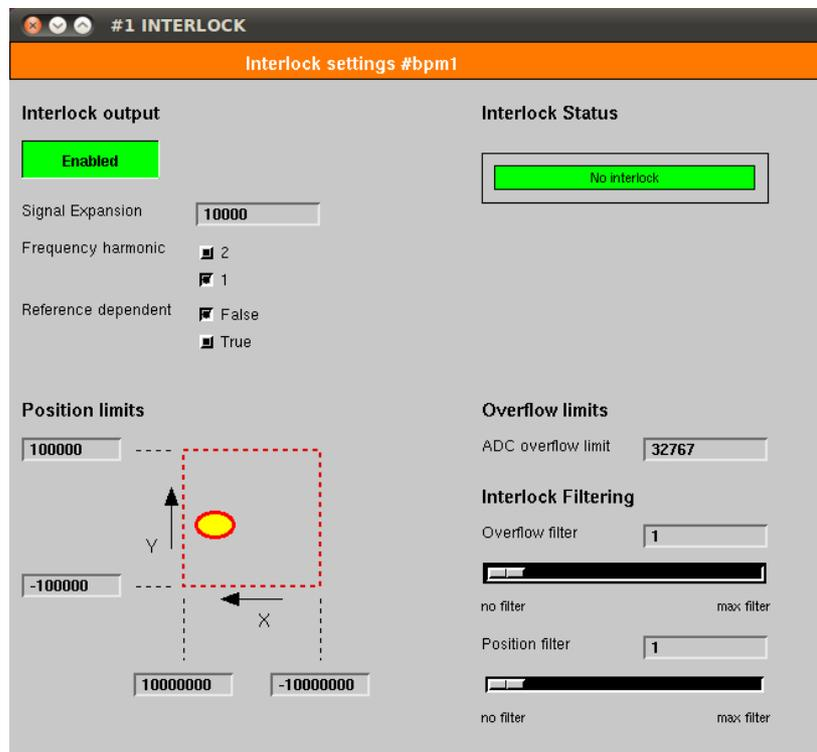
Figure 99: Libera SPH Interlock configuration through GUI
