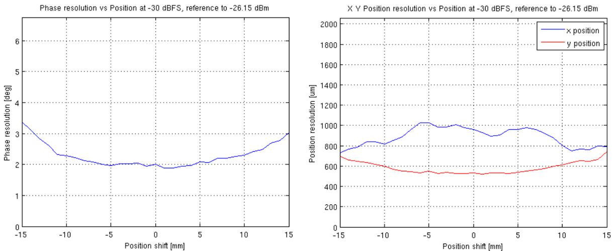
Figure 96: Phase and position resolution vs position at -30dBFS
