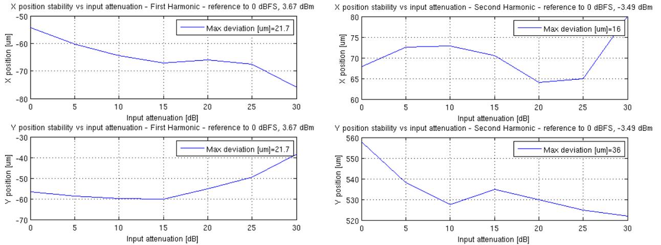
Figure 42: Position stability vs input signal level
