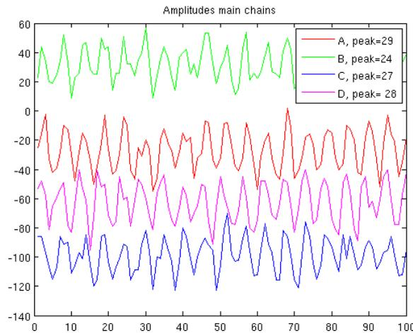
Figure 95: ADC signal levels at -30 dBFS
