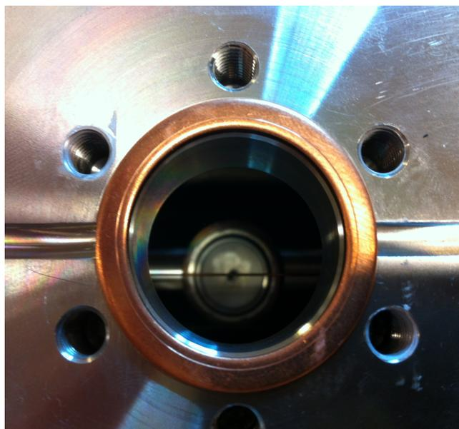
*Figure 3: The wire passing through the BPM*
