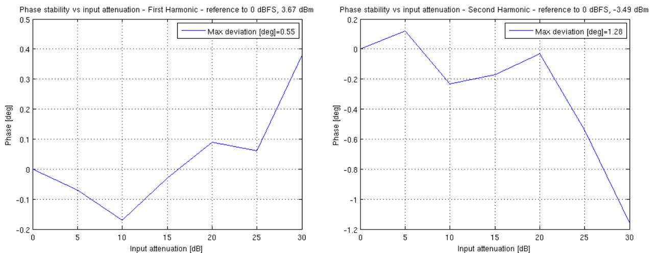
Figure 41: Phase stability vs input signal level
