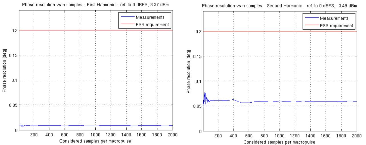
Figure 19: Phase resolution dependence on number of samples per macro-pulse, 0 dBFS
