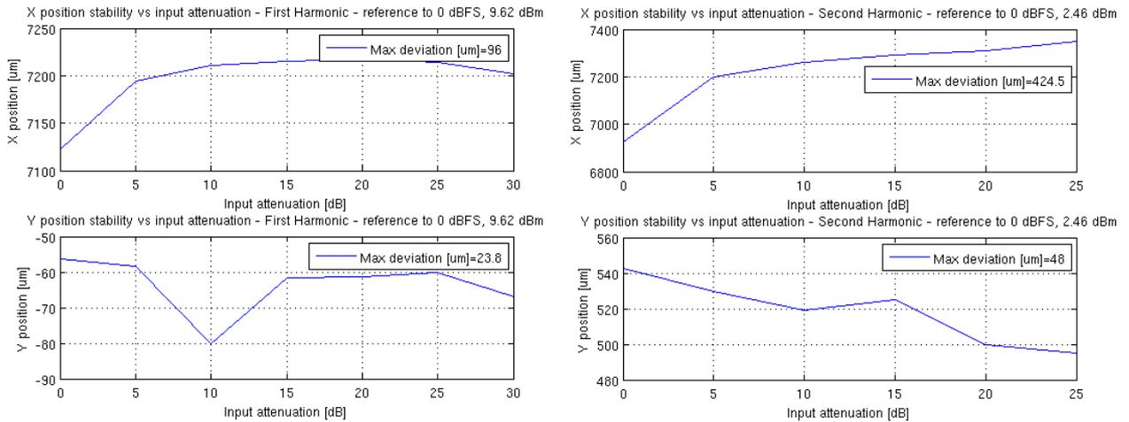
Figure 69: Position stability vs input signal level
