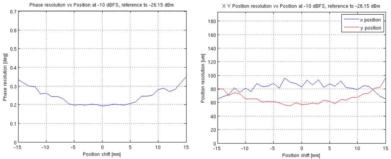
Figure 88: Phase and position resolution vs position at -10dBFS
