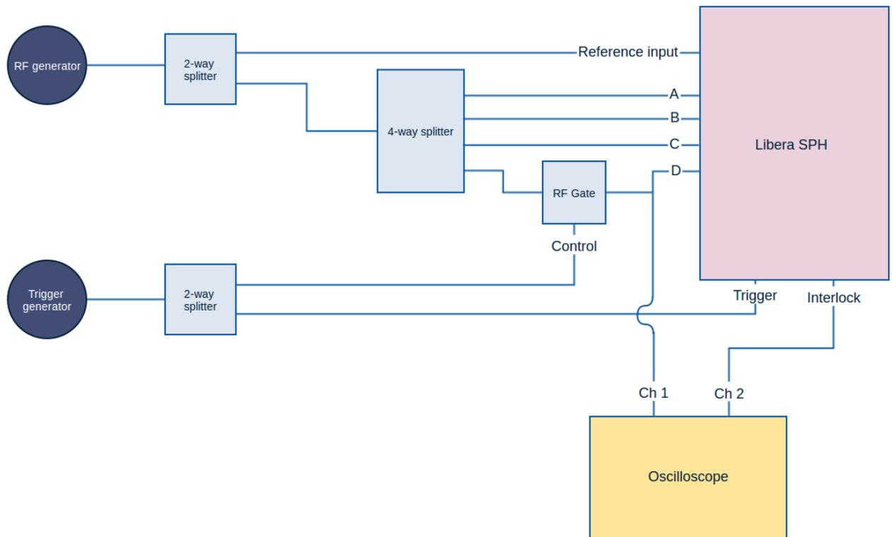
*Figure 100: Setup for the Interlock response time measurement*
