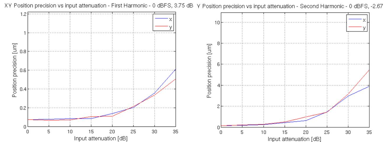
Figure 26: Position precision dependence on the input signal level
