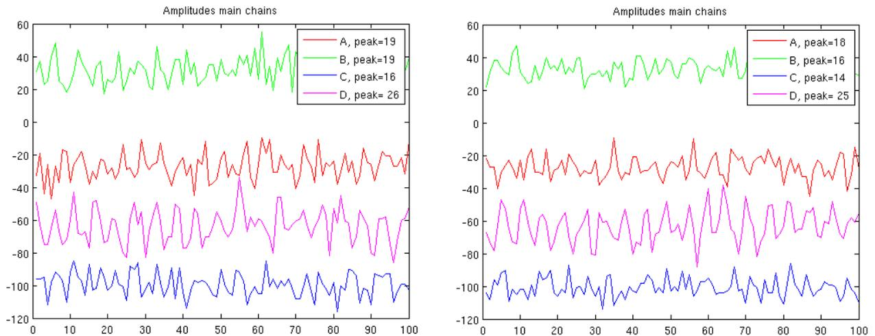
Figure 86: ADC signal acquisitions: a) at -40dBFS b) without RF signal generation
