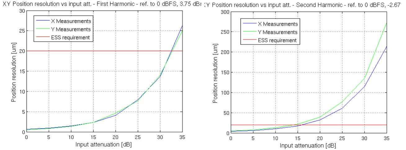
Figure 18: Phase resolution dependence on the input signal level – centered beam
