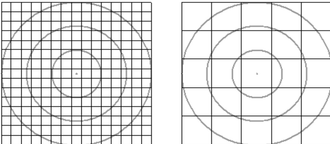
*Figure 5: Resolution dependency on levels of digitization*
