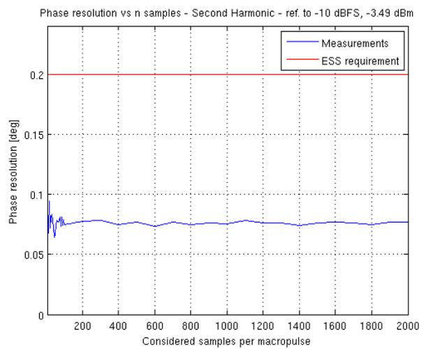
Figure 21: Phase resolution dependence on number of samples per macro-pulse, -10 dBFS
