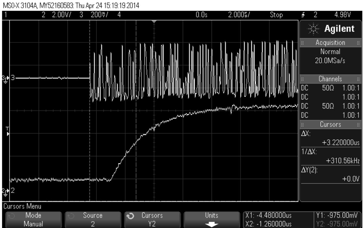
Figure 101: Interlock response time measurement
