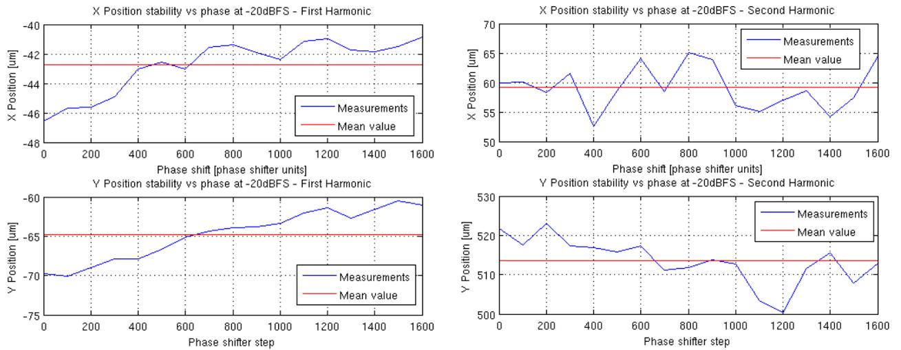
Figure 39: Position stability vs phase at -20dBFS
