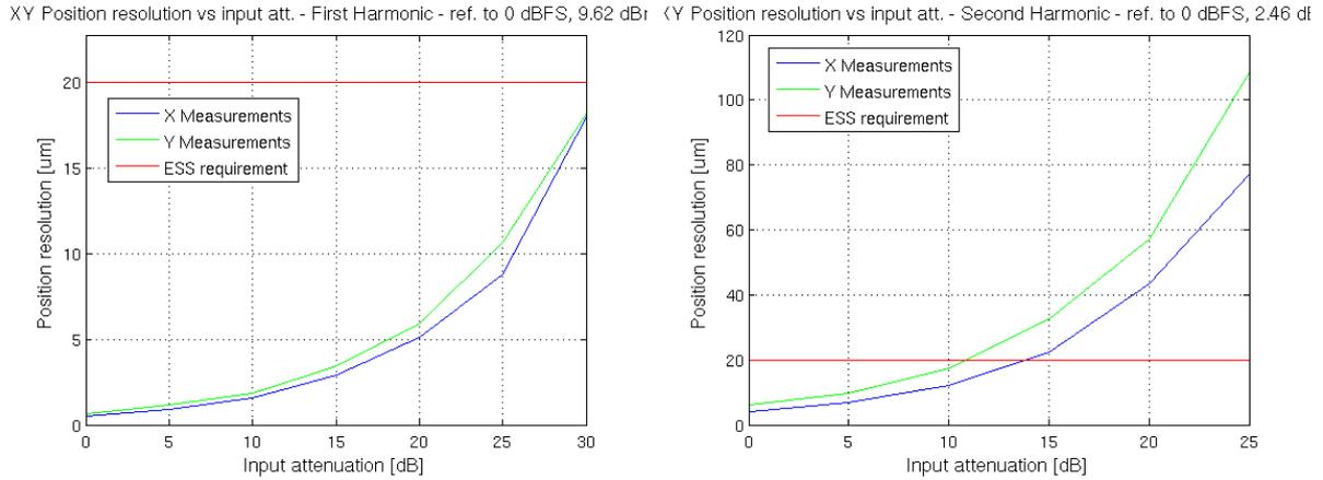
Figure 54: Position resolution dependence on the input signal level – off-centered beam
