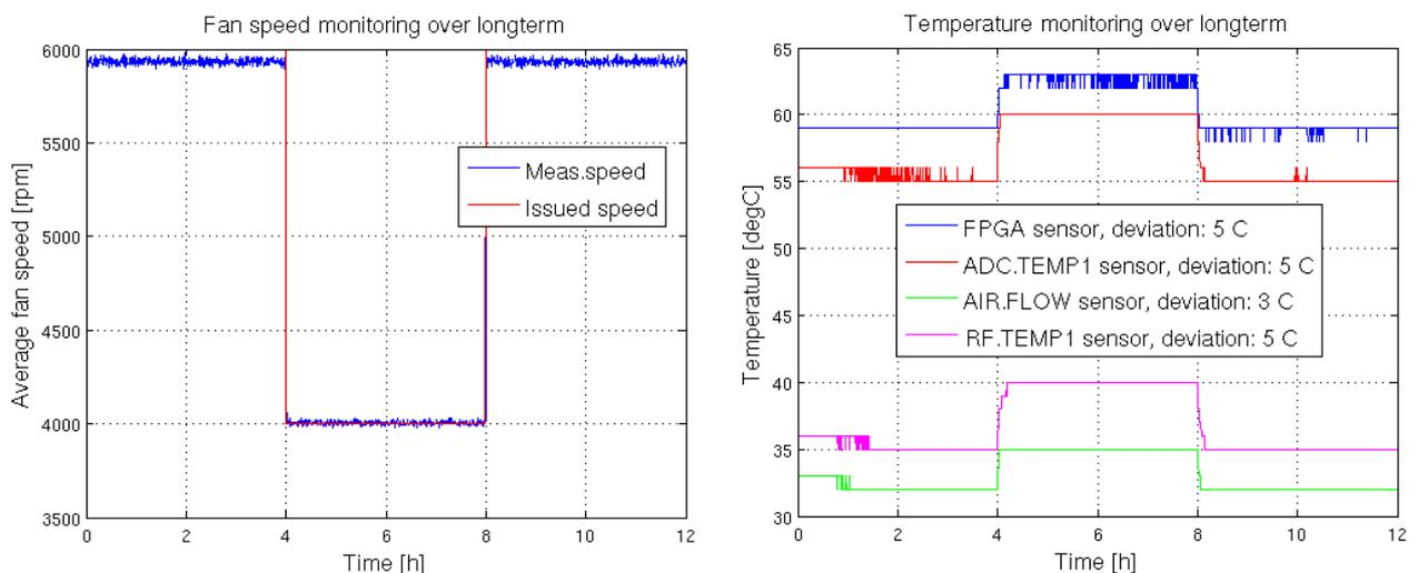
Figure 46: Fans and Temperature change over 12h long-term test
