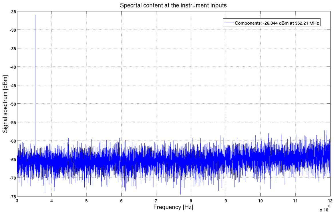
Figure 79: Spectrum of the instrument input signals at 0dBFS
