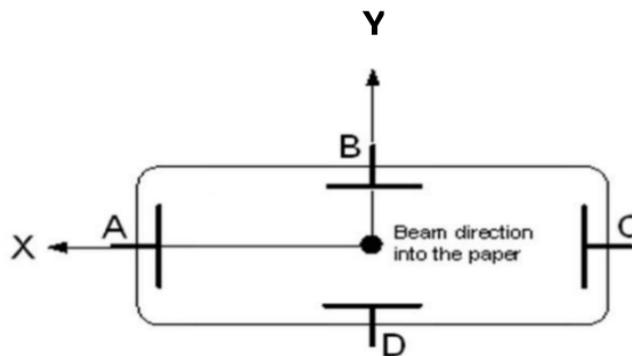
Figure 50: Libera SPH inputs orientation
