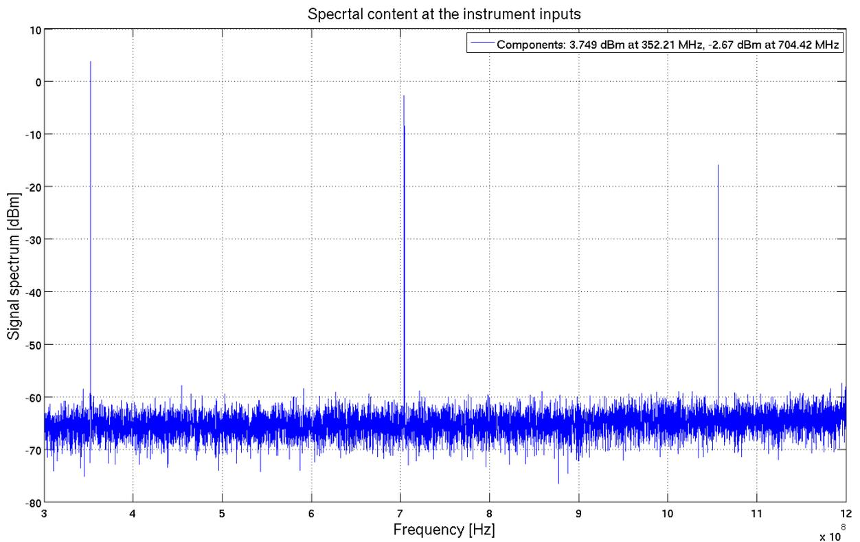
Figure 13: Spectrum of the instrument input signals
