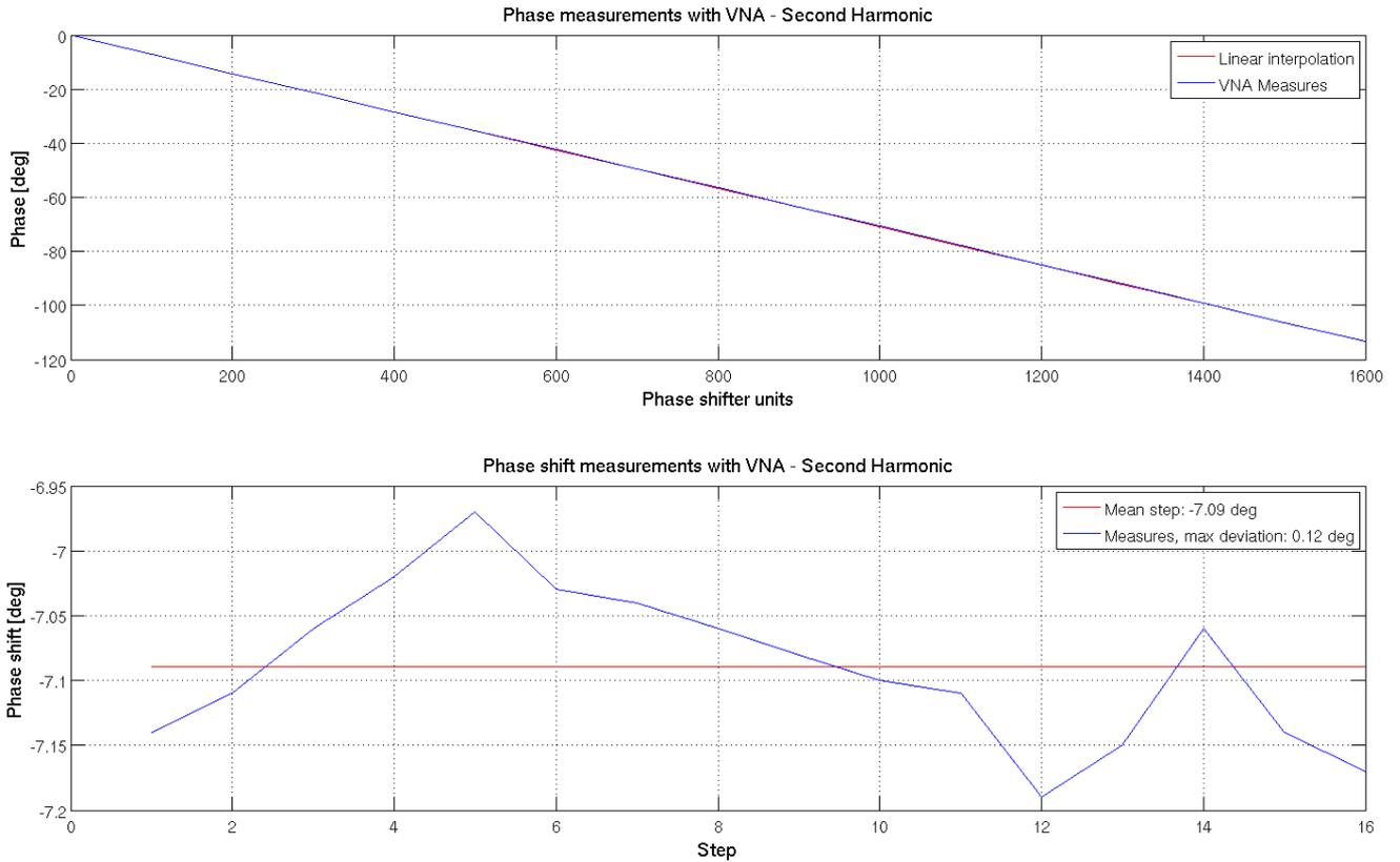
Figure 10: Phase shifter characterization at 704.42 MHz
