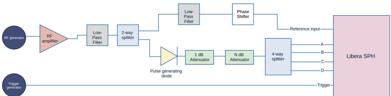
Figure 11: Test setup for measurements with centered beam
