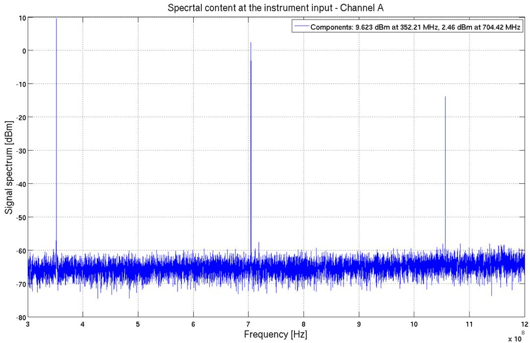
Figure 52: Spectrum of the instrument input signals at 0dBFS
