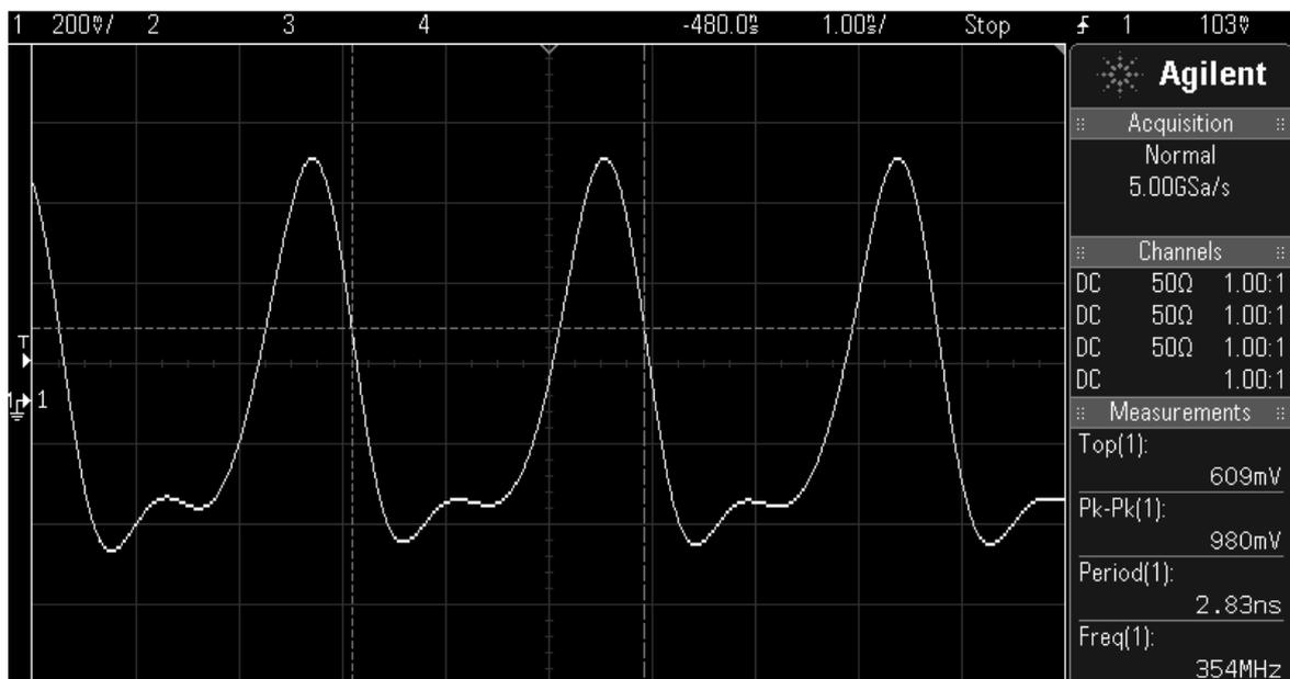
Figure 14: Instrument input signal - time domain
