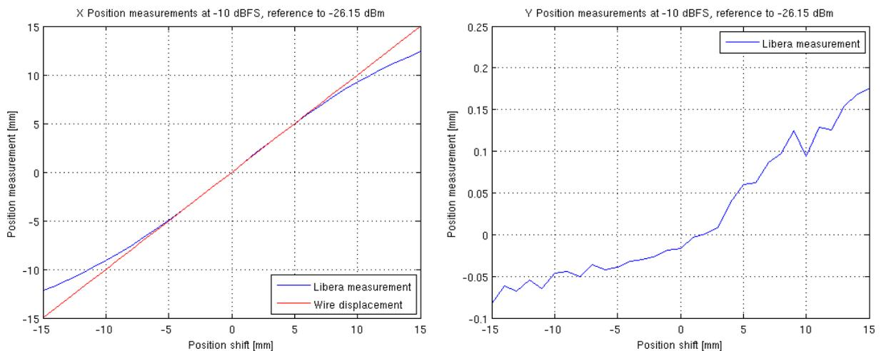
Figure 89: X and Y position measurements at -10dBFS
