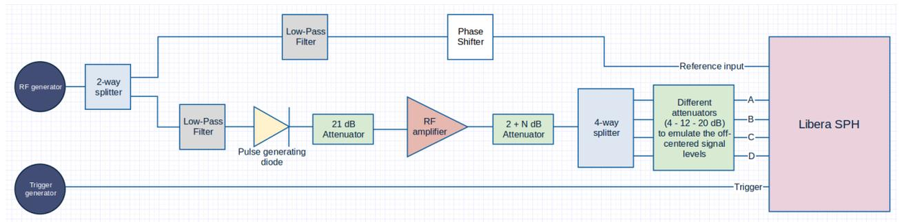
Figure 49: Test setup for measurements with off-centered beam
