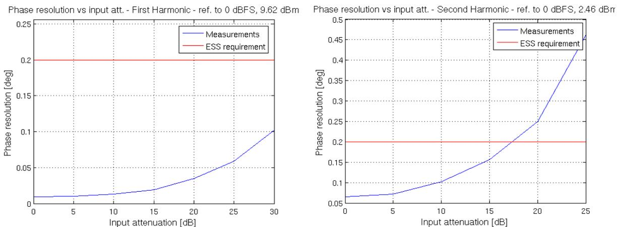
Figure 53: Phase resolution dependence on the input signal level – off-centered beam
