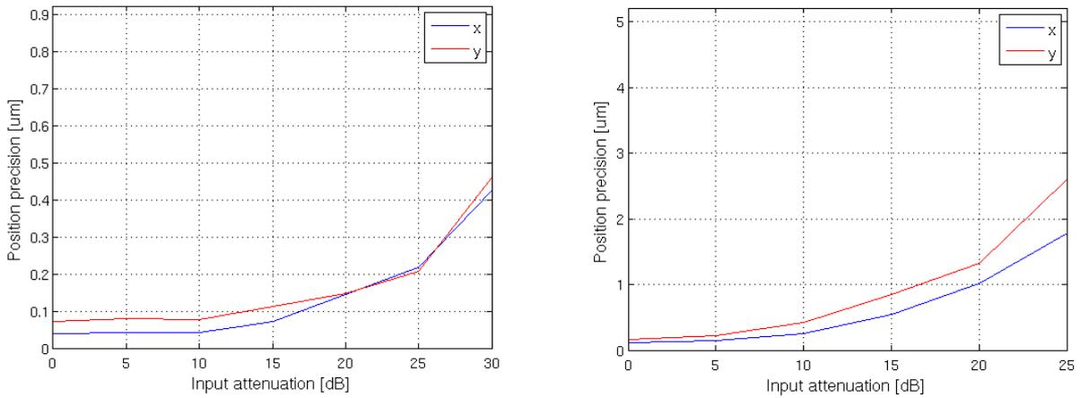
Figure 56: Position precision dependence on the input signal level – off-centered beam
