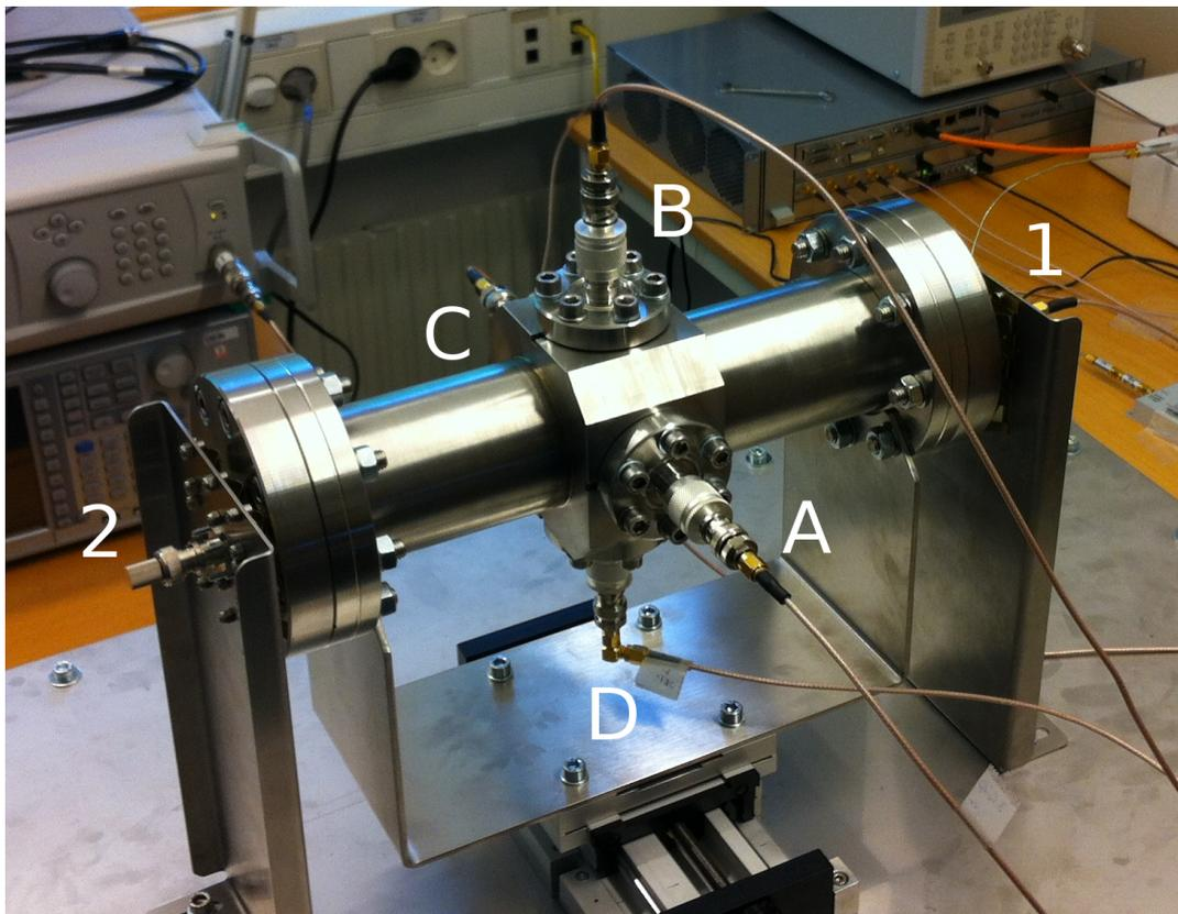
*Figure 70: Port convention for the BPM test-bench*
