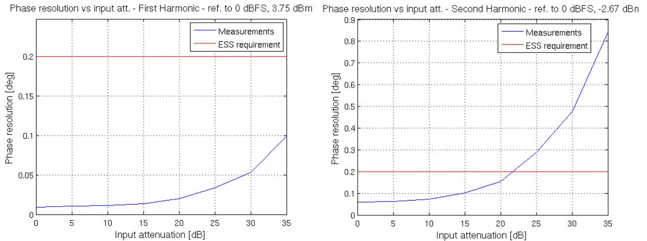
Figure 17: Phase resolution dependence on the input signal level – centered beam
