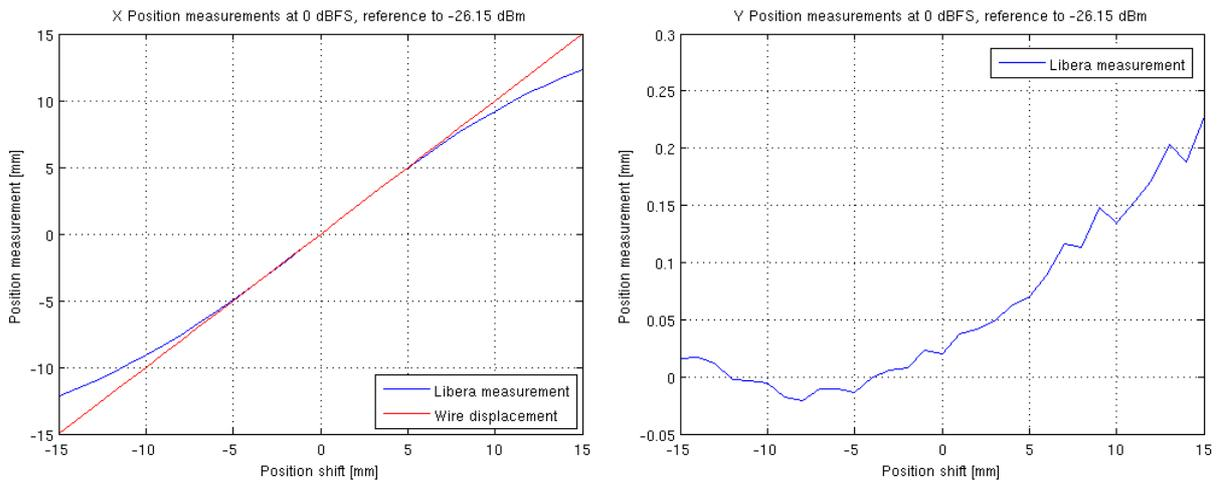
Figure 83: X and Y position measurements at 0dBFS
