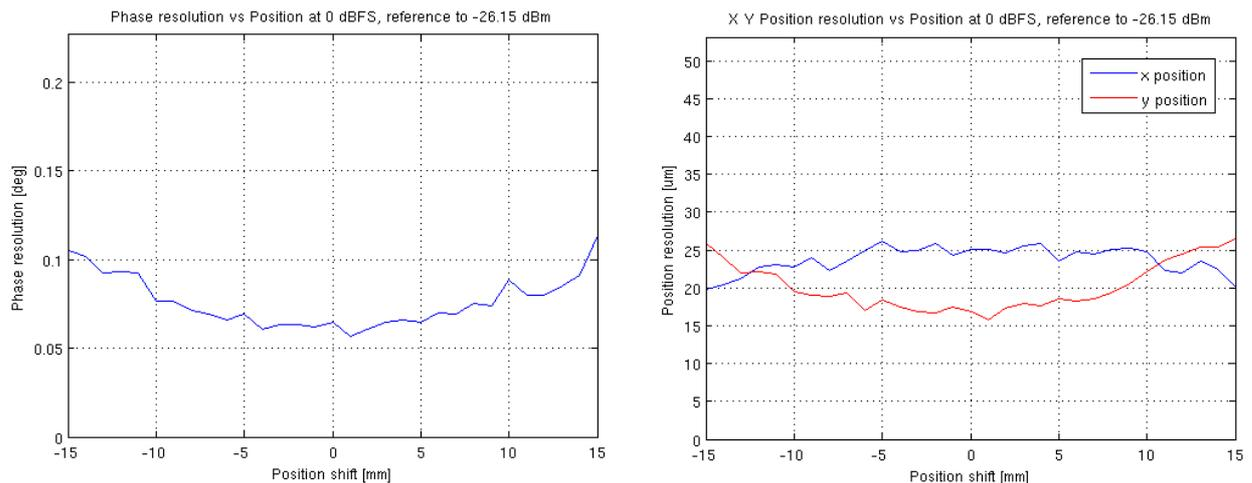
Figure 82: Phase and position resolution vs position at 0dBFS
