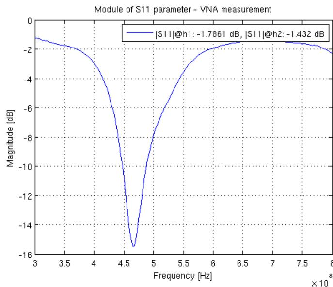
The measurement confirms the bad matching between the RF input (50 Ohm) and the circular waveguide impedance:
