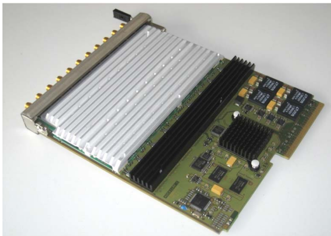
Fig. 3. Bottom view of the 9 channel LLRF receiver double width AMC module
