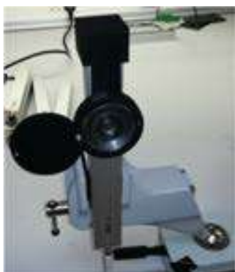
Figure 6: Cesium source positioning on the BLM with a 3D printed support (in black).
