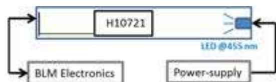
Figure 3: Setup for the calibration with a LED (diode).
