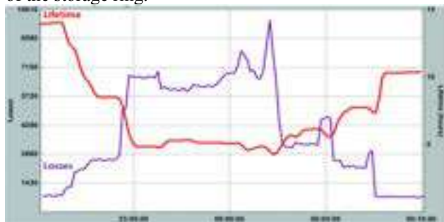
Figure 14: Correlation between losses measurement in slow mode and the beam lifetime.
