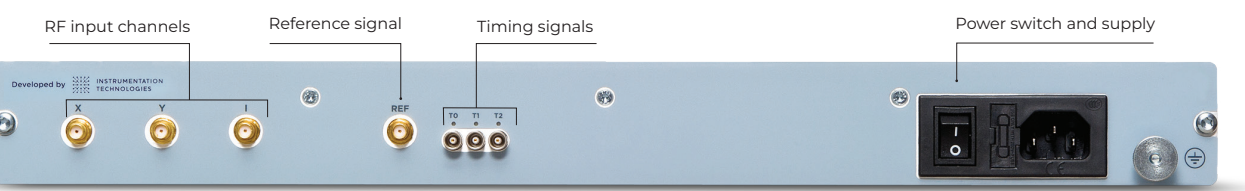
Figure 9: CavityBPM electronics based on Libera integrated platform, back panel
