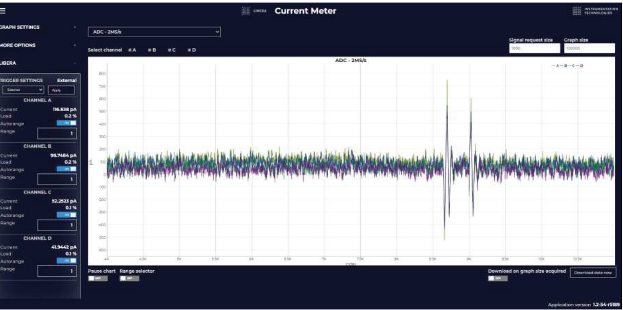
Figure 21: Libera Current Meter Web GUI accessible from web browser
