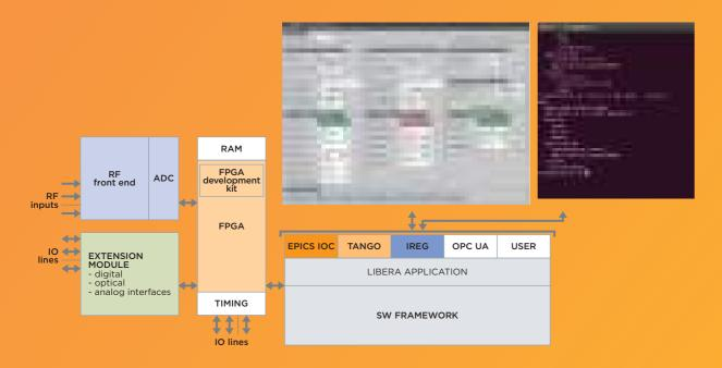
BPM electronics are available in different technology platforms that have different form factors. The BPM modular platform is based on the MTCA.0 modular technology and hosts up to four BPM modules in a 2U 19" chassis. Several extensions are available for the orbit feedback and timing system—see the section on Extensions.
