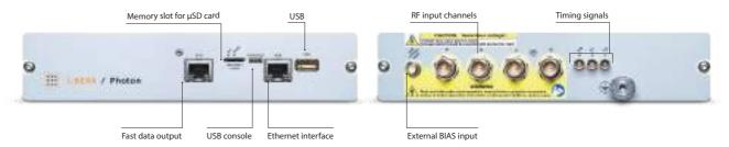
The BPM electronics for the cavity-type BPM pickups are also based on Libera integrated platform, which in this case is enlarged to a 1U 19" chassis due to the higher amount of heat that needs to be passively dissipated. The instrument can be expanded to four RF inputs and SFP connectors for fast data exchange.
