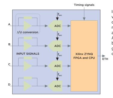
Input currents are converted into voltage via a trans-impedance amplifier, with six different gains depending on the current range selected via software. The signals are then digitized using 18-bit and 2 MSPS A/D converters (sampling frequency can be increased up to 2.5 MSPS). Offsets and gain errors can be calibrated for each channel using a nominal current source.
