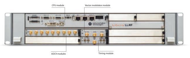
Up to four processing modules (ADC9) can be connected to the system in order to acquire up to 32 RF signals from the cavities; if less signals need to be acquired, the number of ADC9 modules can be reduced.
