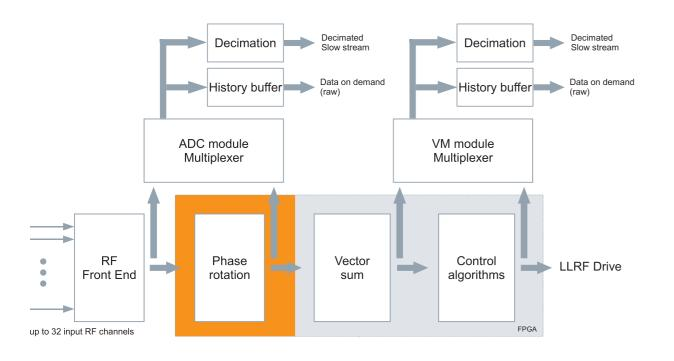
The phase rotation block is used to calibrate each different input signal in phase and amplitude; this is so that differences in RF cabling and delays resulting from the beam time of flight don't influence the calculation. The vector sum then combines all the acquired signals into one equivalent signal, which is used as the input for the control algorithm.
