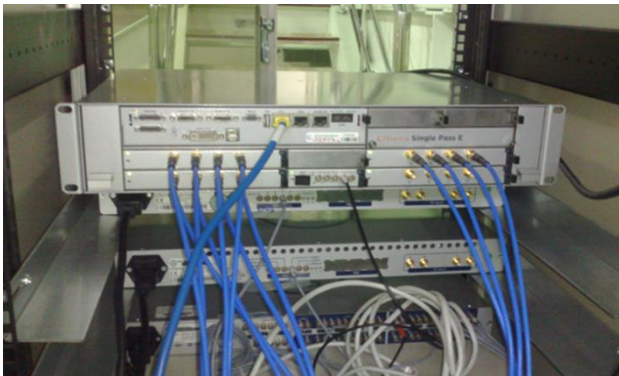
Figure 3: Libera Single Pass E connected to three stripline BPMs
