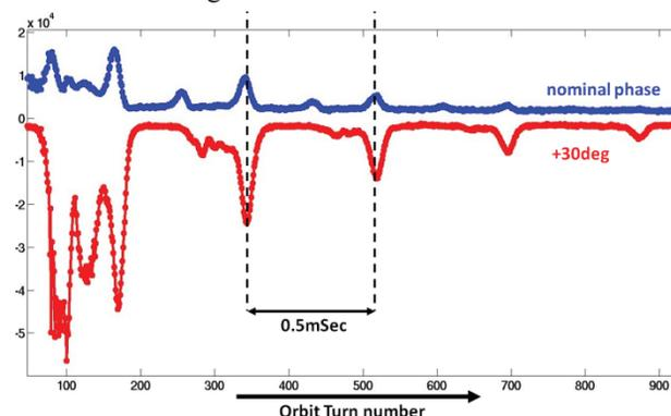
Figure 3: BLD signal at injection, with injected beam at 2 different phases: blue = nominal, red = -30 (plot inverted)
