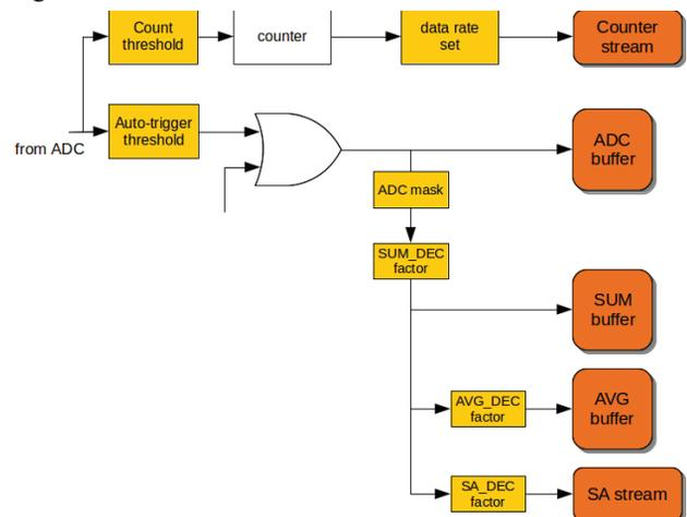
Figure 1: Numeric processing modes in the BLM.
