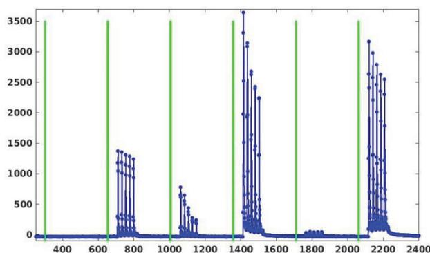
Figure 2: The ADC buffer at injection, showing the injection of the 5 bunches over 6 consecutive turns.
