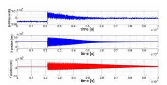
Figure 6: Injection as seen in the turn-by-turn data.
