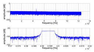
Figure 8: Excitation around betatron frequency.
