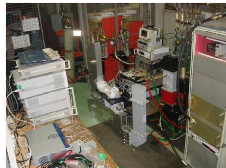
Figure 1: EMMA NS FFAG test setup, Libera LLRF on the table - bottom left corner of the picture
