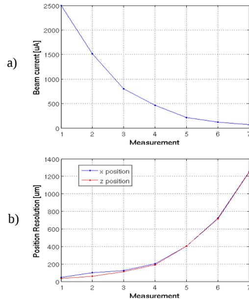
Figure 3.a: current measurements with the SUM signal; Figure 3.b: X and Z position resolution Vs current.
