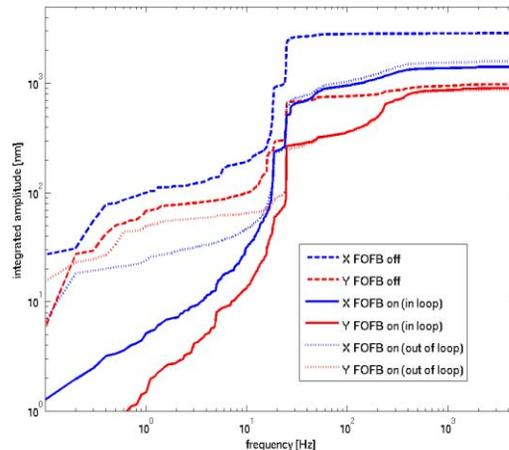
Figure 4: Comparison of integrated amplitude of positional noise for horizontal (X) and vertical (Y) with loop control on and off
