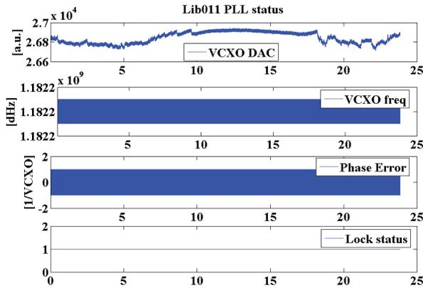
Figure 4: PLL stability during 24 hours.
