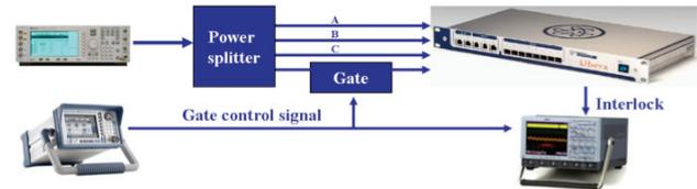
Figure 5: Test setup for latency measurements
