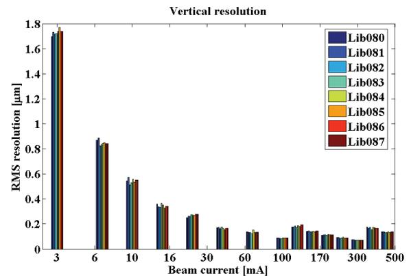
Figure 2: Vertical resolution of 8 Liberass @ 10kHz rate
