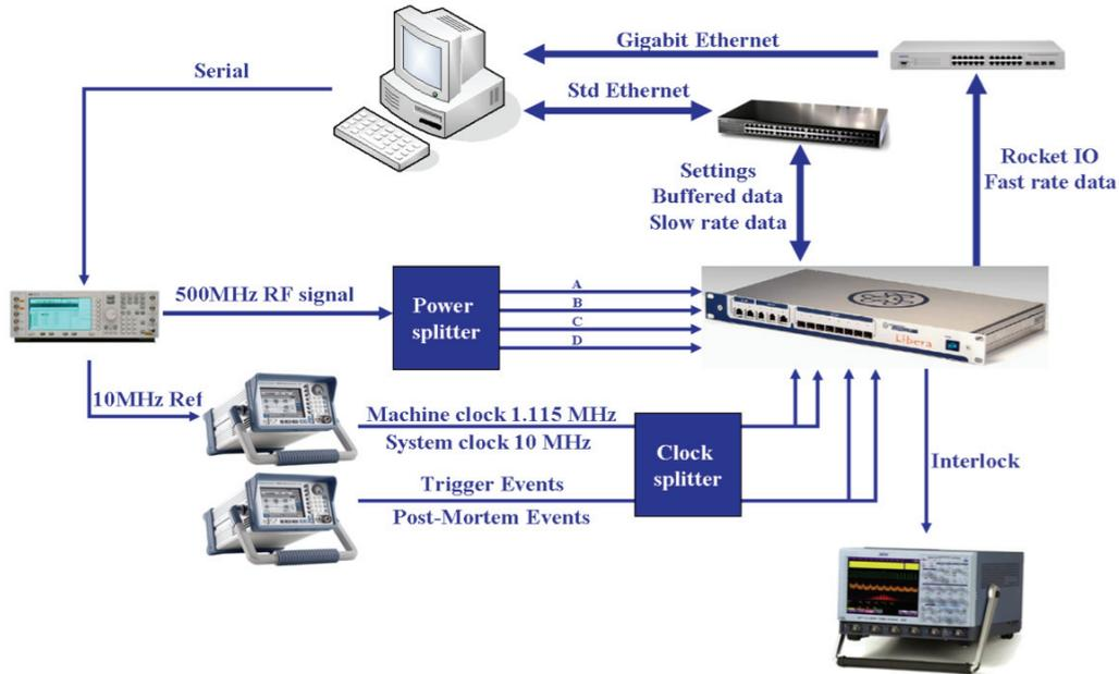
Figure 1: Laboratory test setup for Liberas measurements
