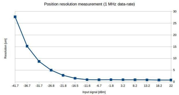
Figure 6: Macro-pulse measurement performance versus input signal level (0 dBFS = 22 dBm).
