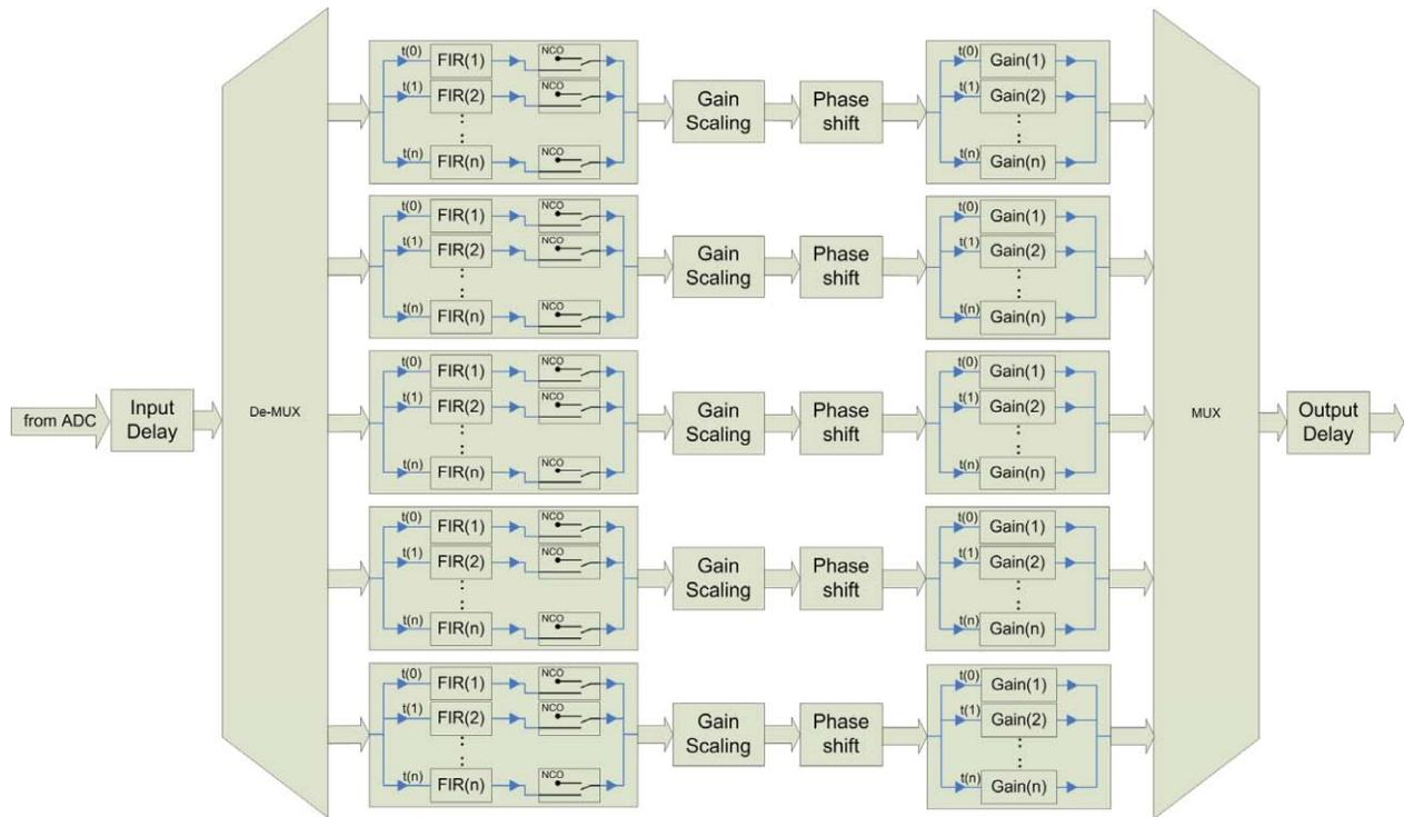
Figure 2: Digital Signal Processing block.
