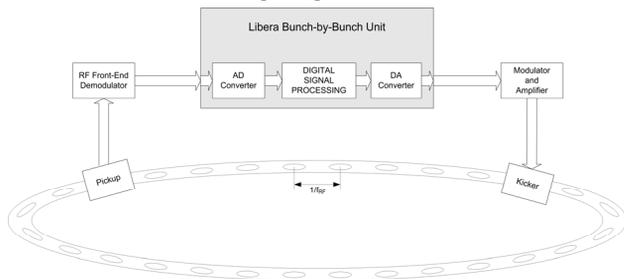
Figure 1: Simplified Bunch-by-Bunch feedback scheme.
