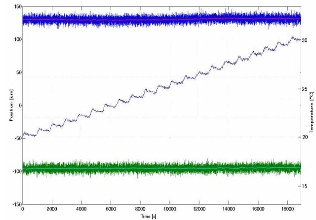
Figure 5: X and Y position (Red and Light Blue are Averaged Values) during temperature stability test
