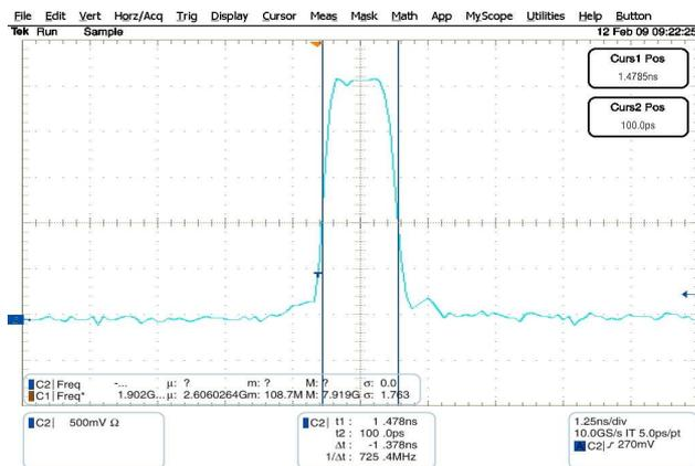
Figure 3: Simulated Signal Seen Through 15 dB Attenuator
