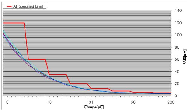
**Figure 7: RMS Results Measured on Four Libera Brilliance Single Pass Units. FAT Limits are depicted with Blue Line.**
