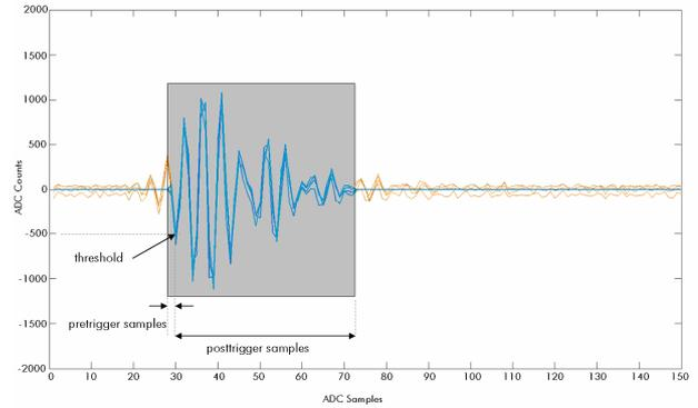
**Figure 2: Parameter Definition for Single Pass Position Calculation**
